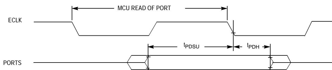
**Figure 63 Port Read Timing Diagram**
