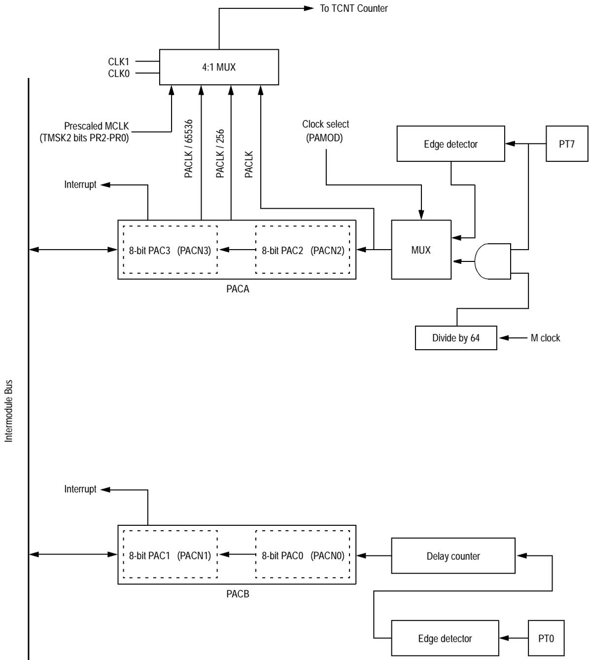
**Figure 29 16-Bit Pulse Accumulators Block Diagram**
