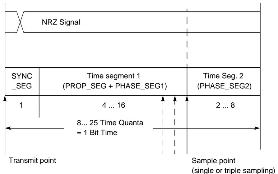
**Figure 49 Segments within the Bit Time**
