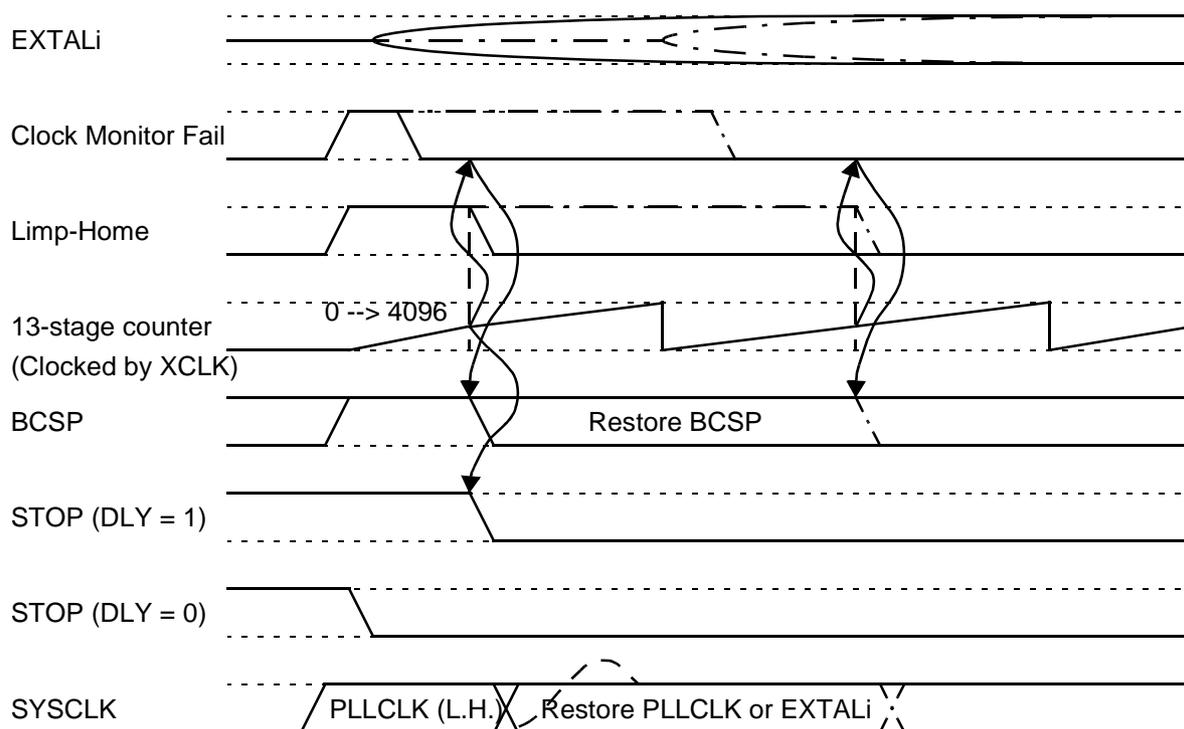
**Figure 18 STOP Exit and Fast STOP Recovery**
