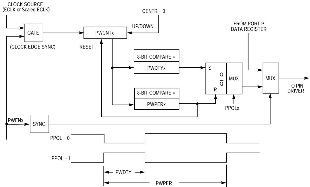
**Figure 23 Block Diagram of PWM Left-Aligned Output Channel**
