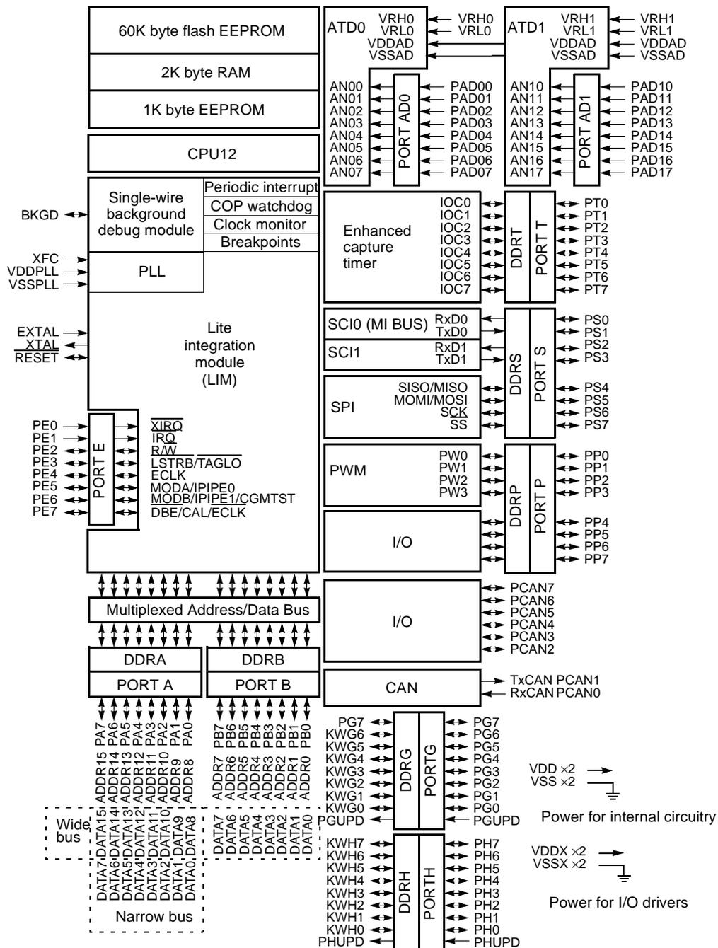
Figure 1 MC68HC912D60A 112-pin QFP Block Diagram
