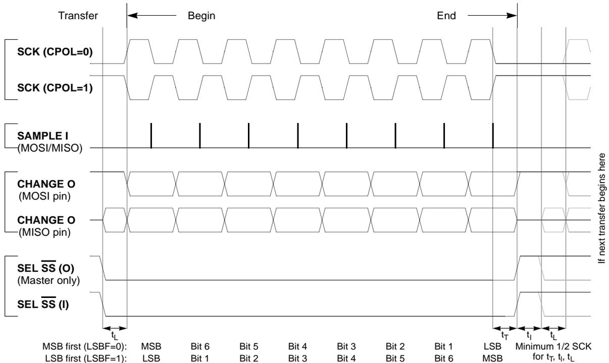
**Figure 36 SPI Clock Format 1 (CPHA = 1)**
