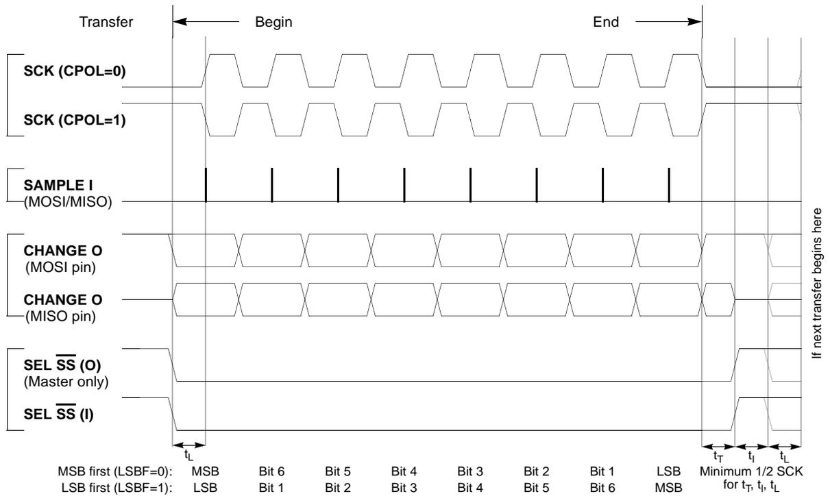
**Figure 35 SPI Clock Format 0 (CPHA = 0)**
