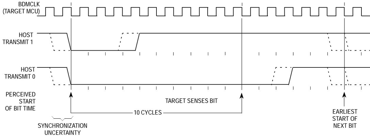
**Figure 55 BDM Host to Target Serial Bit Timing**
