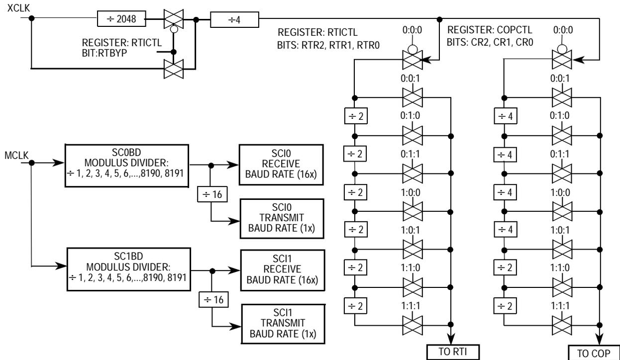
**Figure 20 Clock Chain for SCI0, SCI1, RTI, COP**
