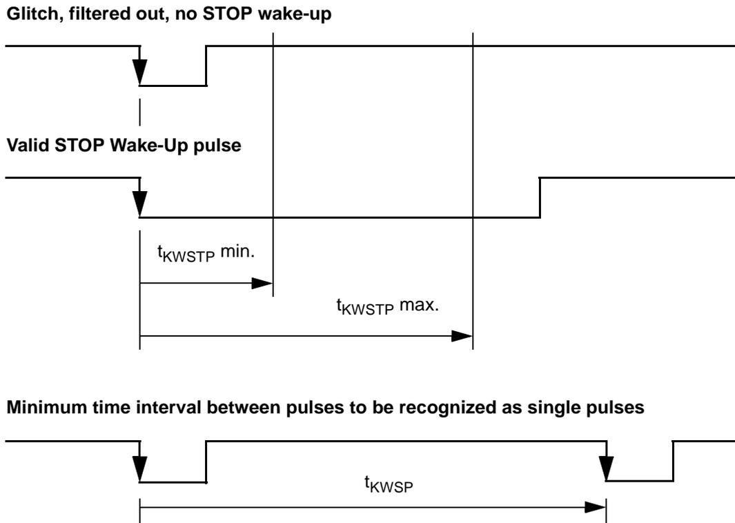
**Figure 13 STOP Key Wake-up Filter (falling edge trigger) timing**
