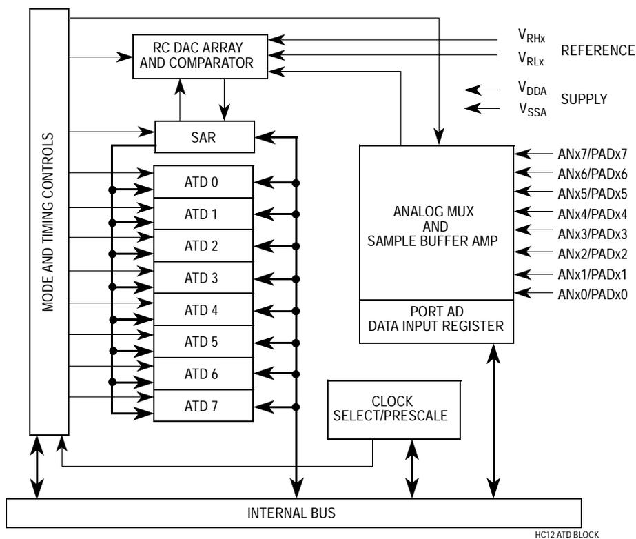
**Figure 54 Analog-to-Digital Converter Block Diagram**
