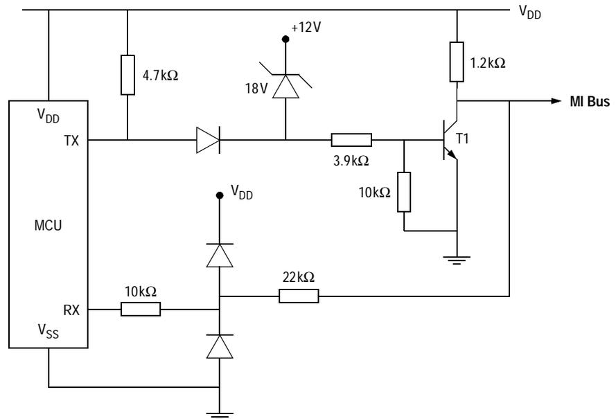
**Figure 41 A typical MI Bus interface**
