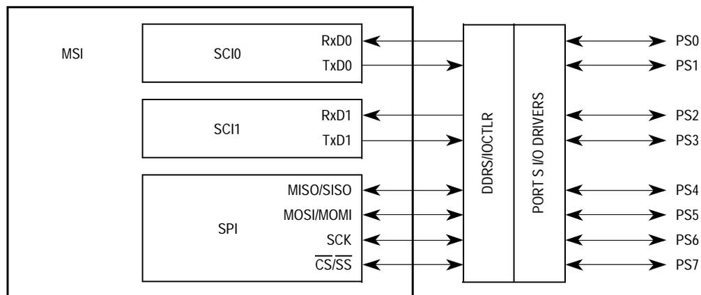
**Figure 32 Multiple Serial Interface Block Diagram**
