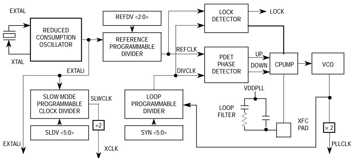
**Figure 15 PLL Functional Diagram**
