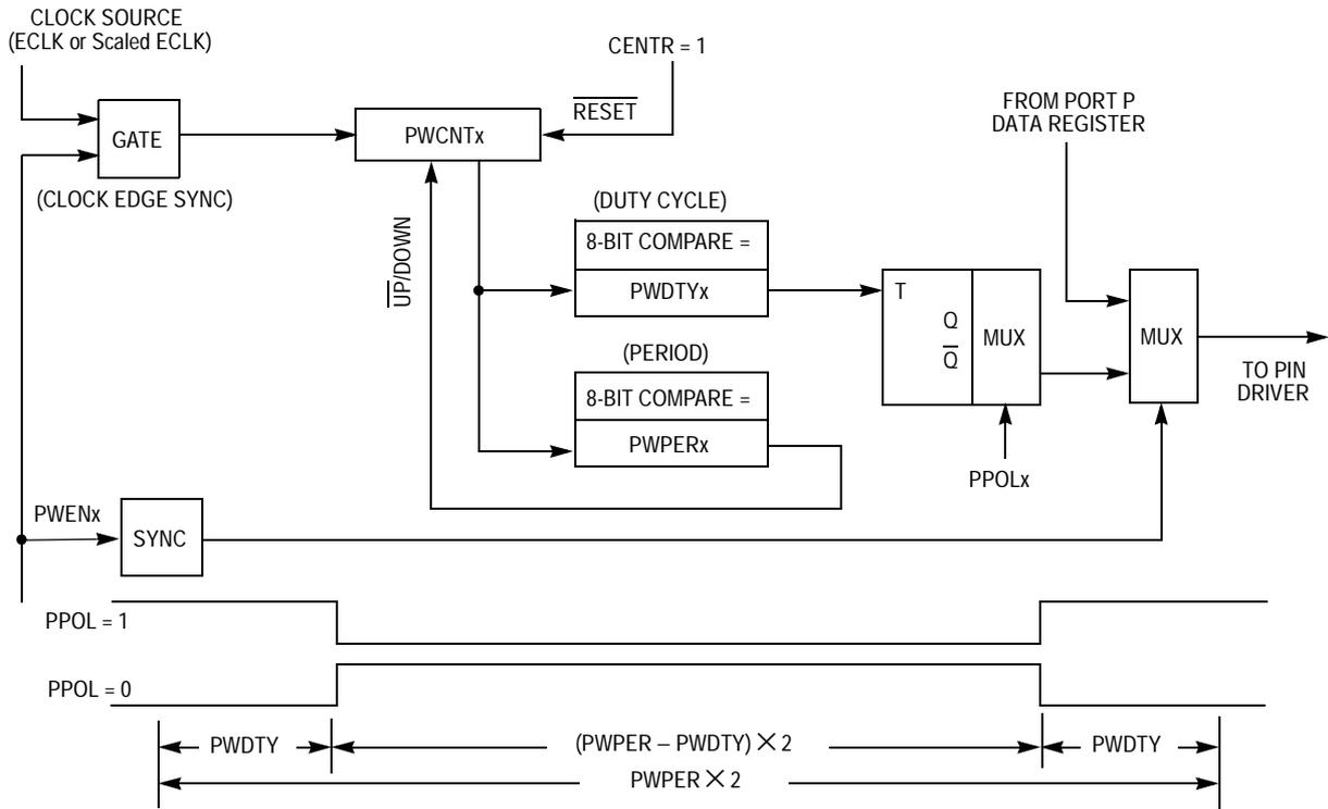
**Figure 24 Block Diagram of PWM Center-Aligned Output Channel**
