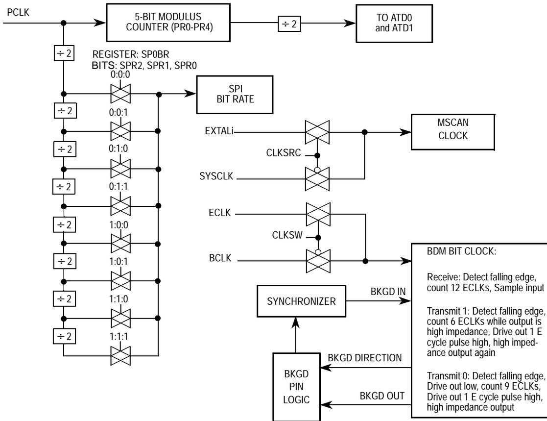
**Figure 22 Clock Chain for MSCAN, SPI, ATD0, ATD1 and BDM**
