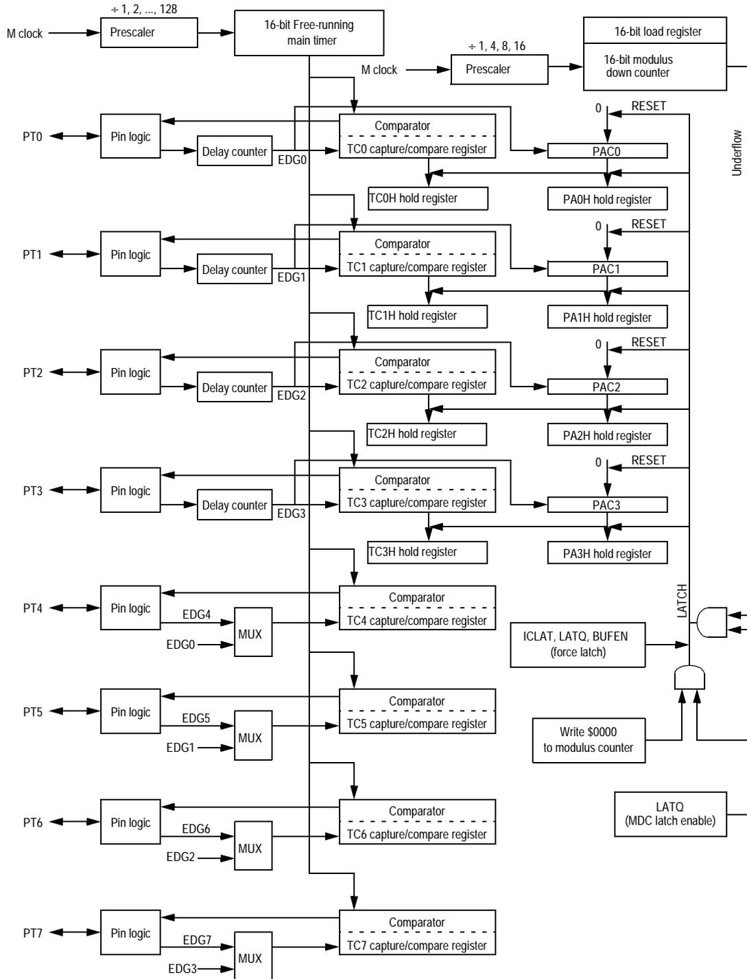
**Figure 26 Timer Block Diagram in Latch Mode**
