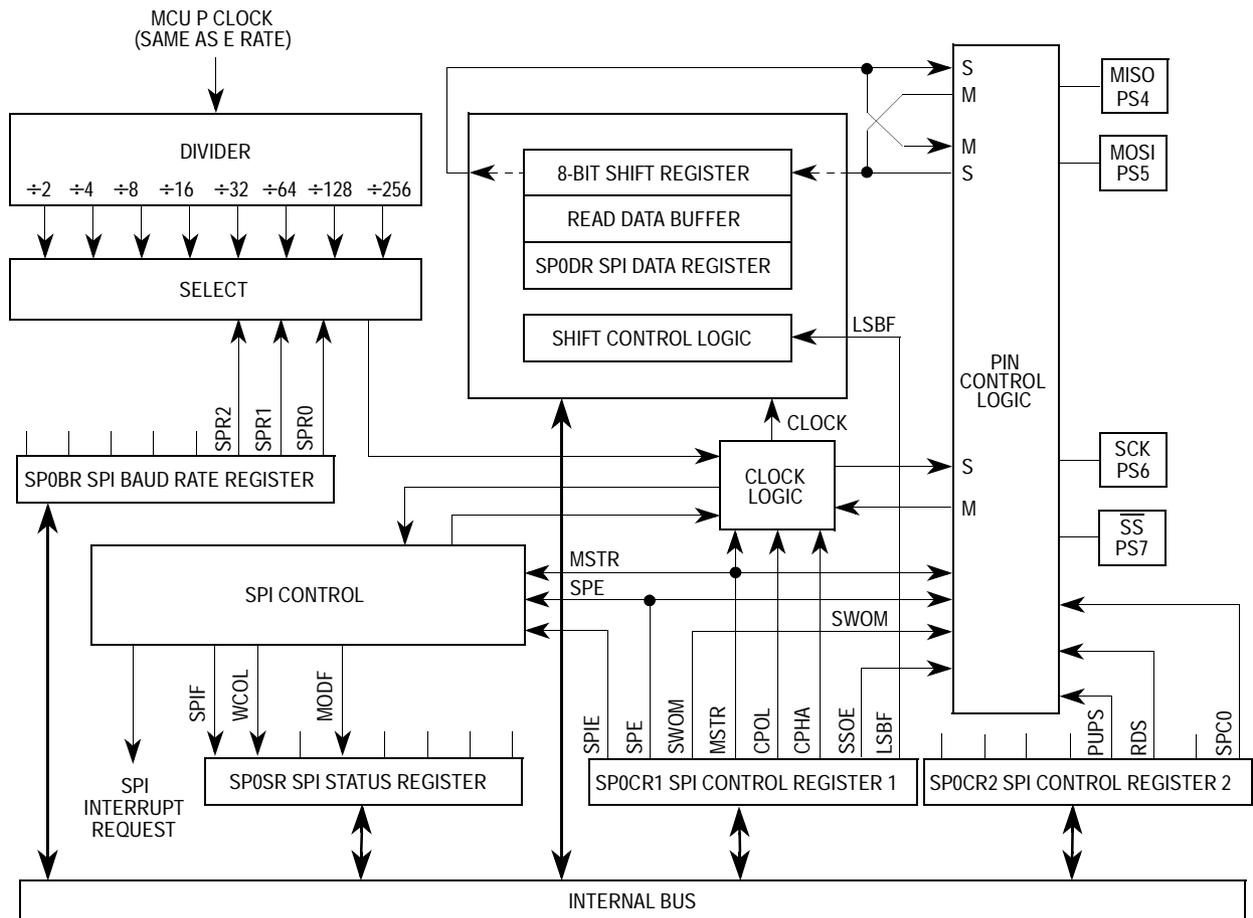
**Figure 34 Serial Peripheral Interface Block Diagram**
