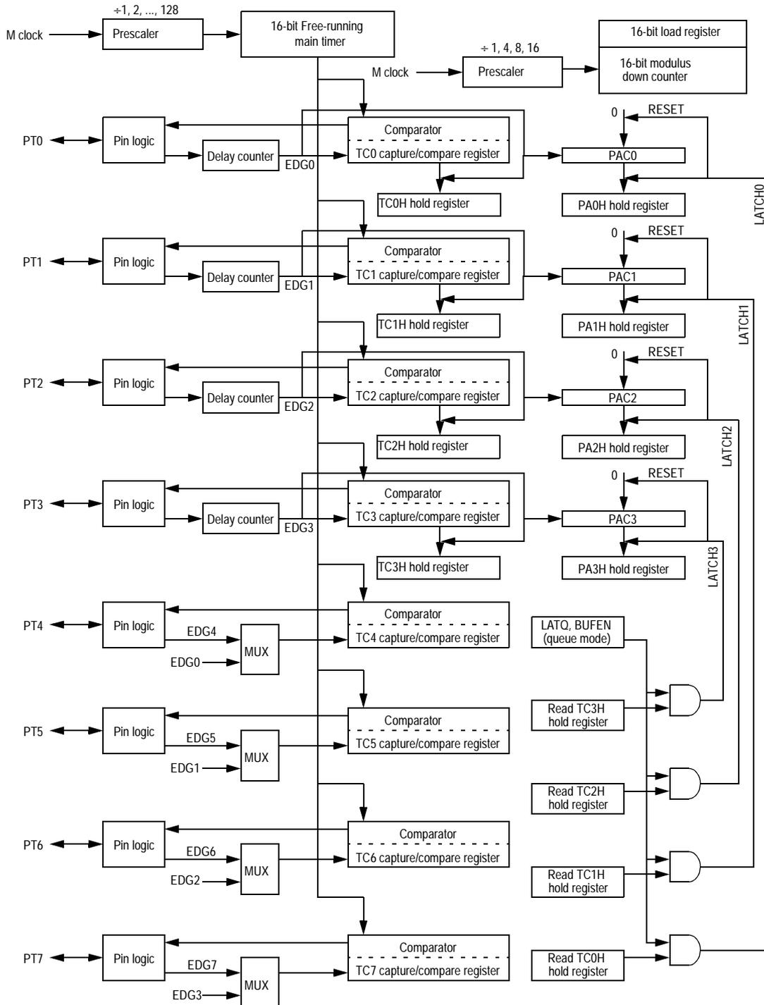
**Figure 27 Timer Block Diagram in Queue Mode**
