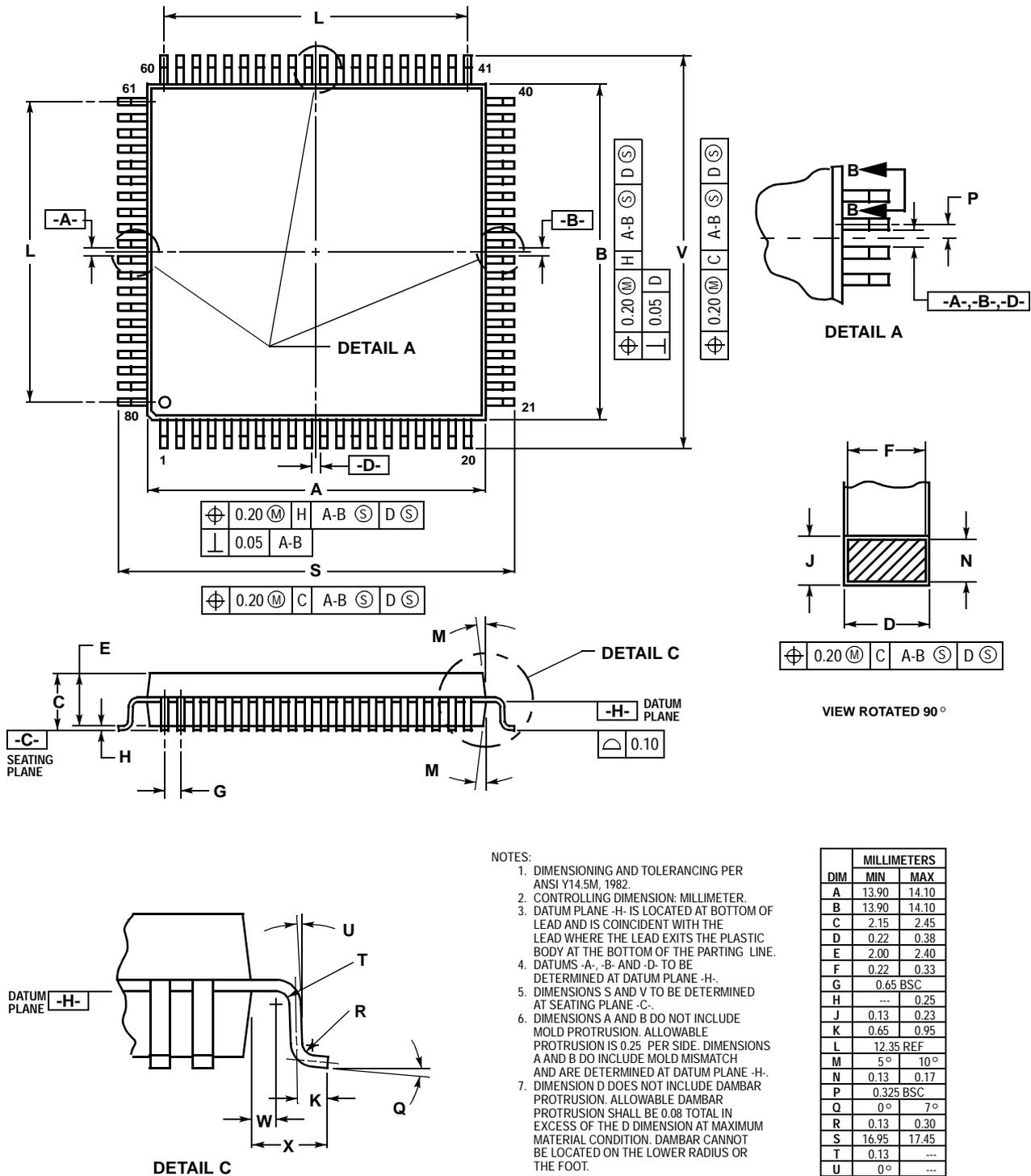
Figure 7 80-pin QFP Mechanical Dimensions (case no. 841B)
