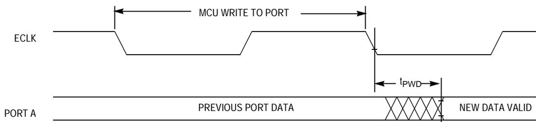
**Figure 64 Port Write Timing Diagram**
