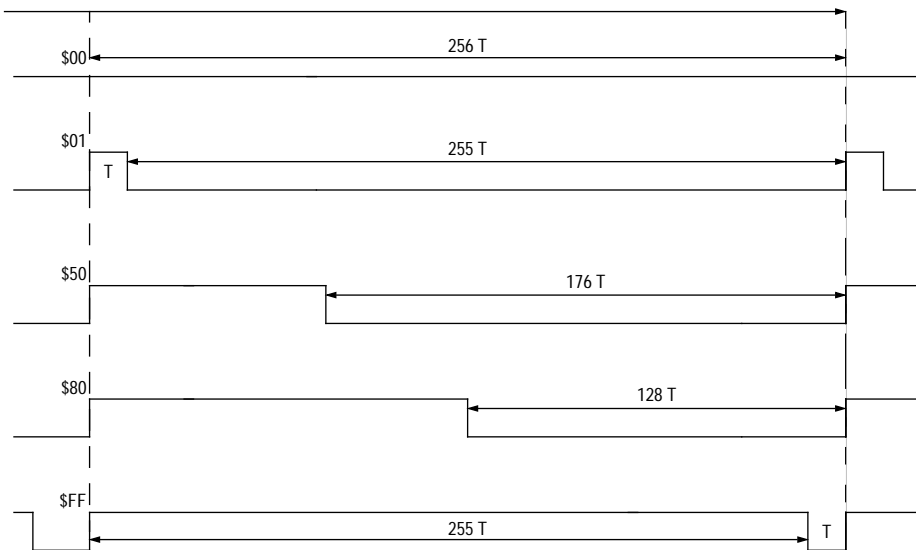
Figure 12-2 PWM output waveforms (POL = 1, active high)
