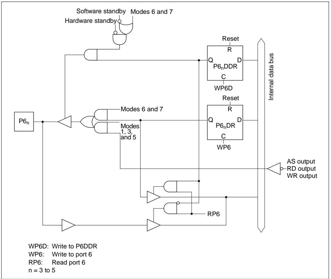
**Figure C-5 (b) Port 6 Block Diagram (Pins P6<sub>3</sub> to P6<sub>5</sub>)**
