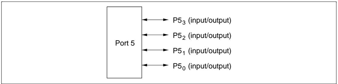
**Figure 7-15 Pin Functions in Mode 7 (Port 5)**
