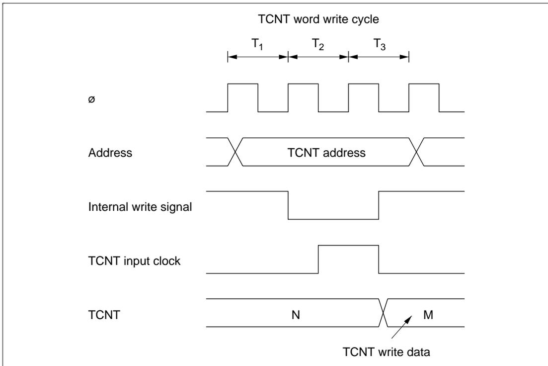
**Figure 8-62 Contention between TCNT Word Write and Increment**
