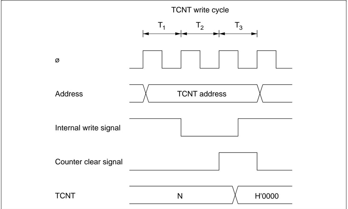
**Figure 8-61** Contention between TCNT Write and Clear
