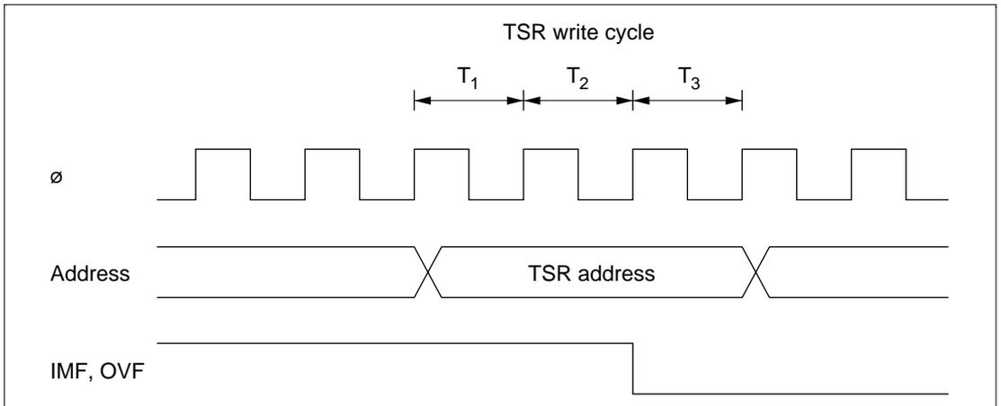
**Figure 8-60 Timing of Clearing of Status Flags**
