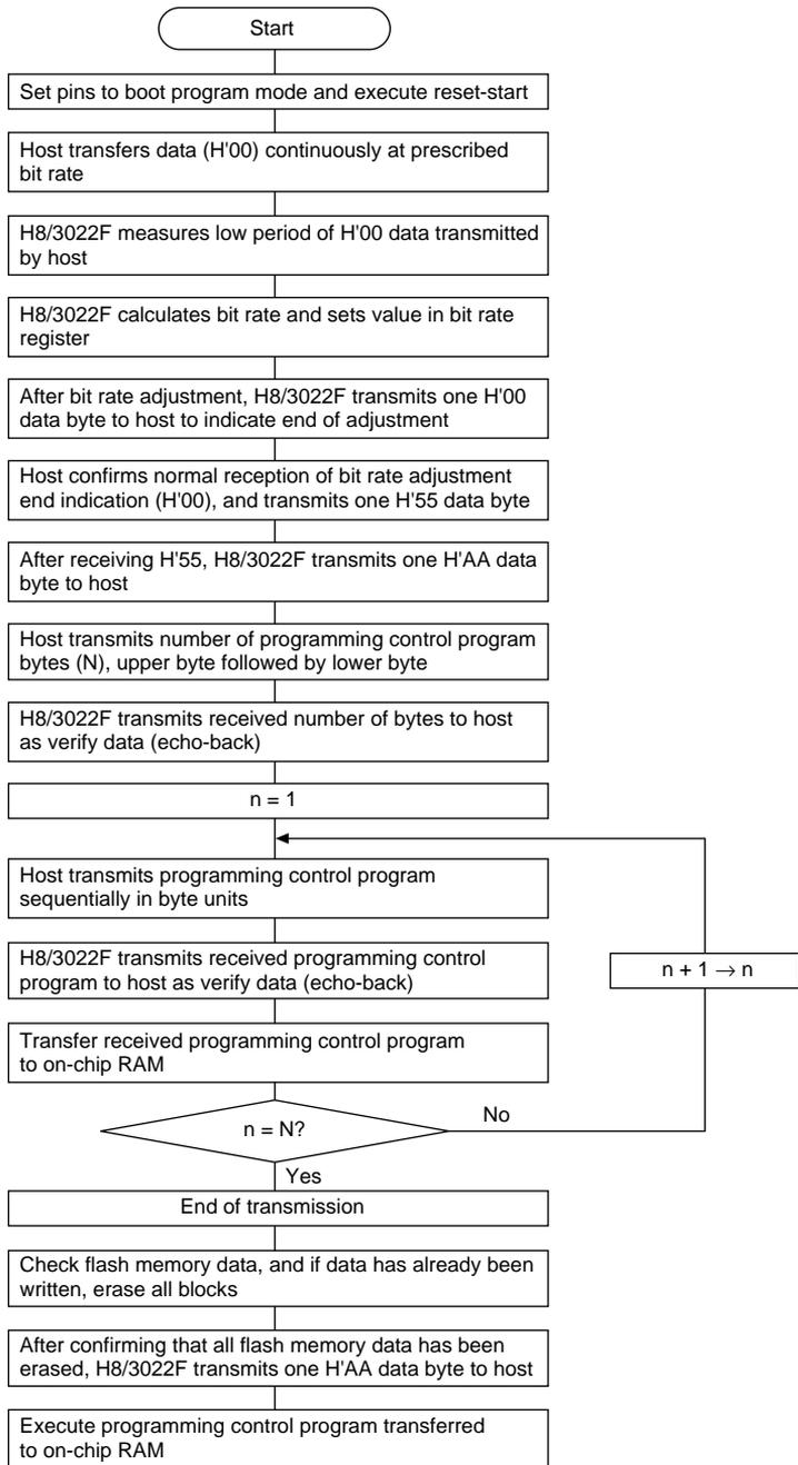
Note: If a memory cell malfunctions and cannot be erased, the H8/3022F sends one H'FF byte as an erase error, and stops the erase operation and subsequent operations.
