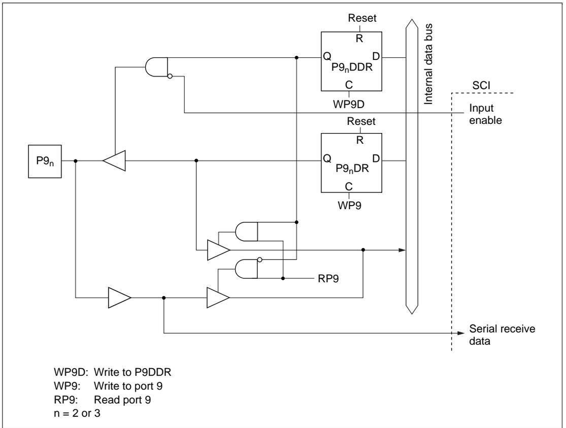
**Figure C-8 (c) Port 9 Block Diagram (Pins P9<sub>2</sub> and P9<sub>3</sub>)**
