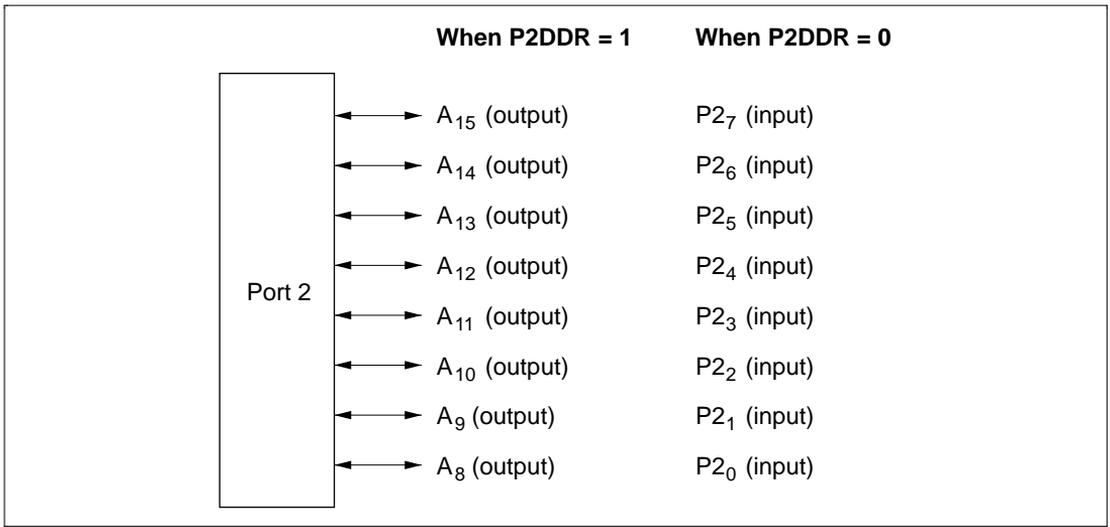
**Figure 7-7 Pin Functions in Modes 5 and 6 (Port 2)**
