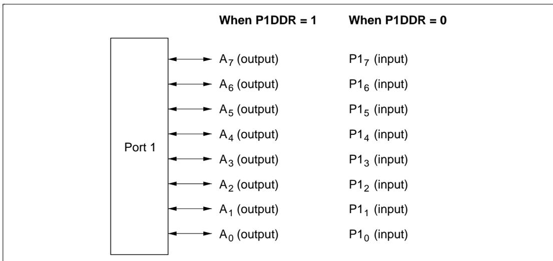
**Figure 7-3 Pin Functions in Modes 5 and 6 (Port 1)**
