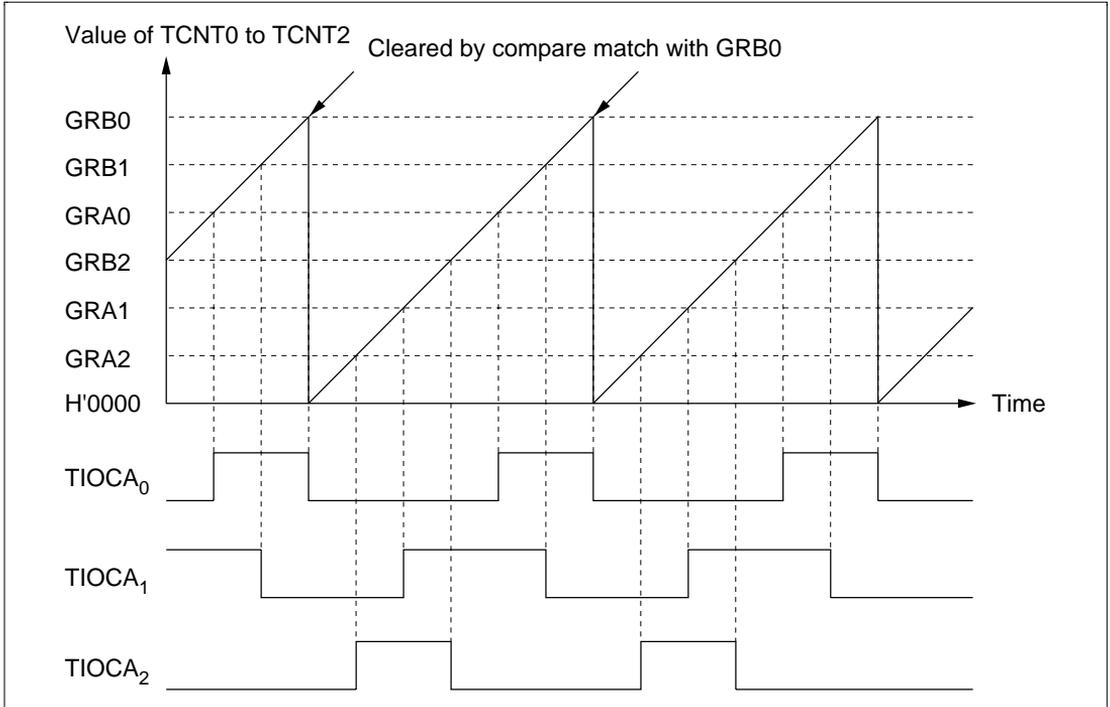
**Figure 8-27 Synchronization (Example)**
