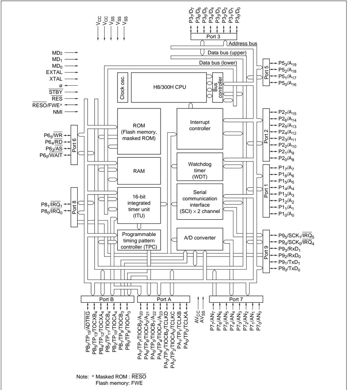
Figure 1-1 Block Diagram
