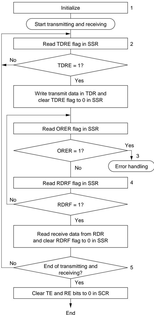
1. SCI initialization: the transmit data output function of the TxD pin and receive data input function of the RxD pin are selected, enabling simultaneous transmitting and receiving.
