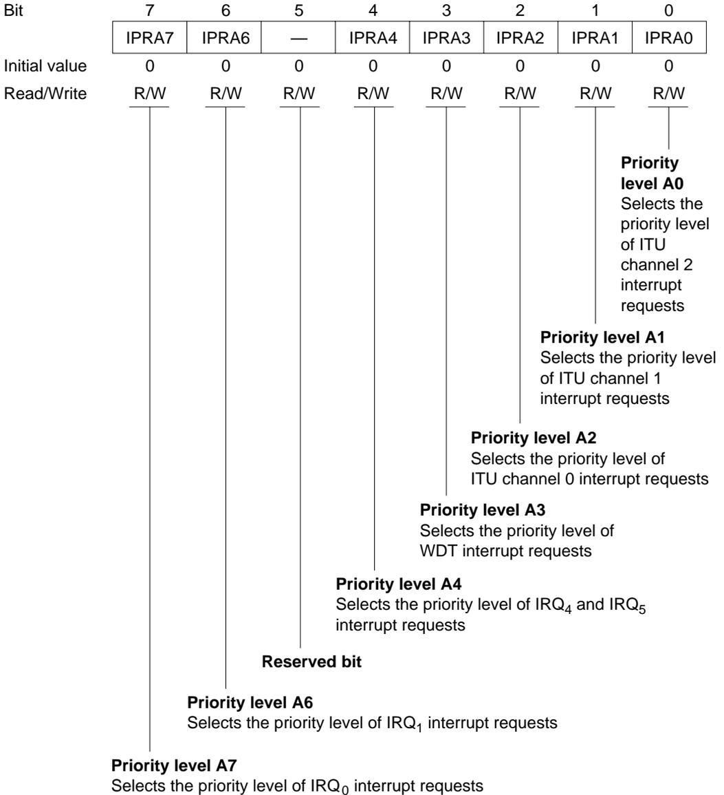
IPRA is initialized to H'00 by a reset and in hardware standby mode.
