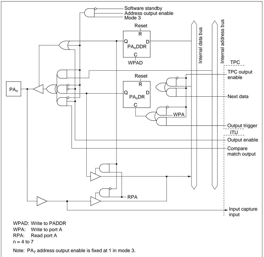
**Figure C-9 (c) Port A Block Diagram (Pins PA<sub>4</sub> to PA<sub>7</sub>)**
