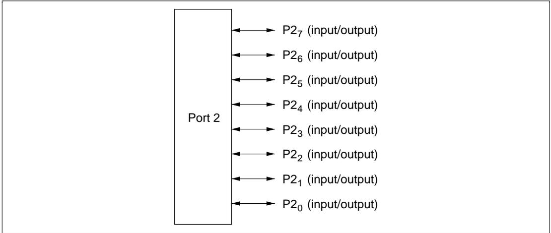
**Figure 7-8 Pin Functions in Mode 7 (Port 2)**
