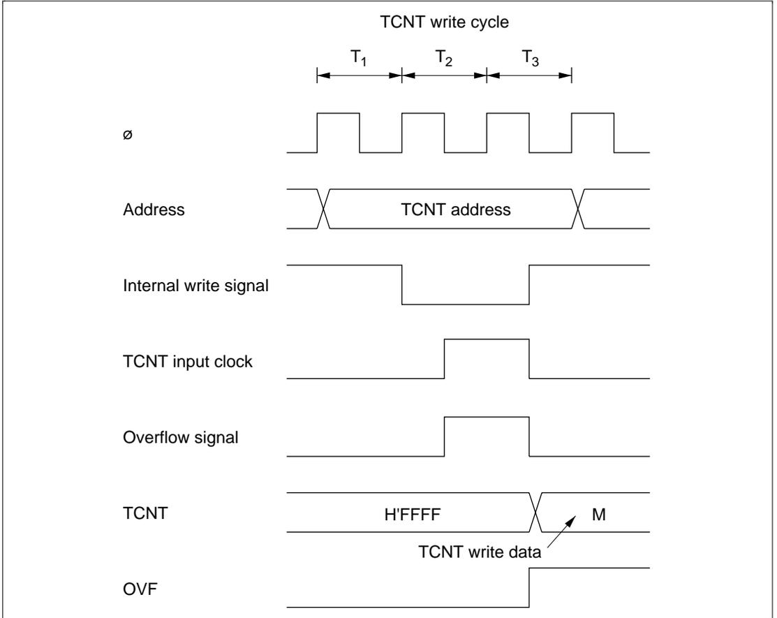
**Figure 8-65 Contention between TCNT Write and Overflow**
