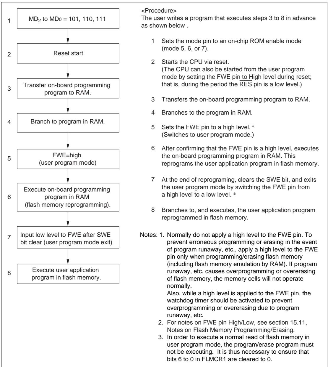
**Figure 15-9 User Program Mode Execution Procedure (Example)**
