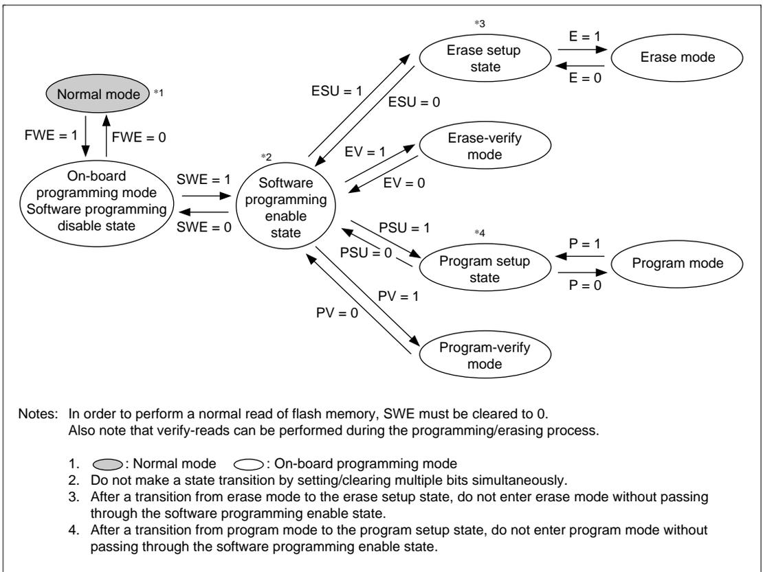
**Figure 15-10 State Transitions Caused by FLMCR1 Bit Settings**
