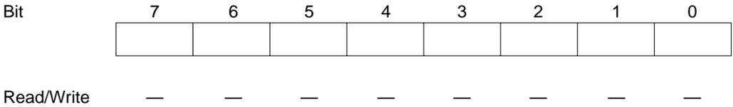
The SCI loads transmit data from TDR into TSR, then transmits the data serially from the TxD pin, LSB (bit 0) first. After transmitting one data byte, the SCI automatically loads the next transmit data from TDR into TSR and starts transmitting it. If the TDRE flag is set to 1 in SSR, however, the SCI does not load the TDR contents into TSR. The CPU cannot read or write TSR directly.
