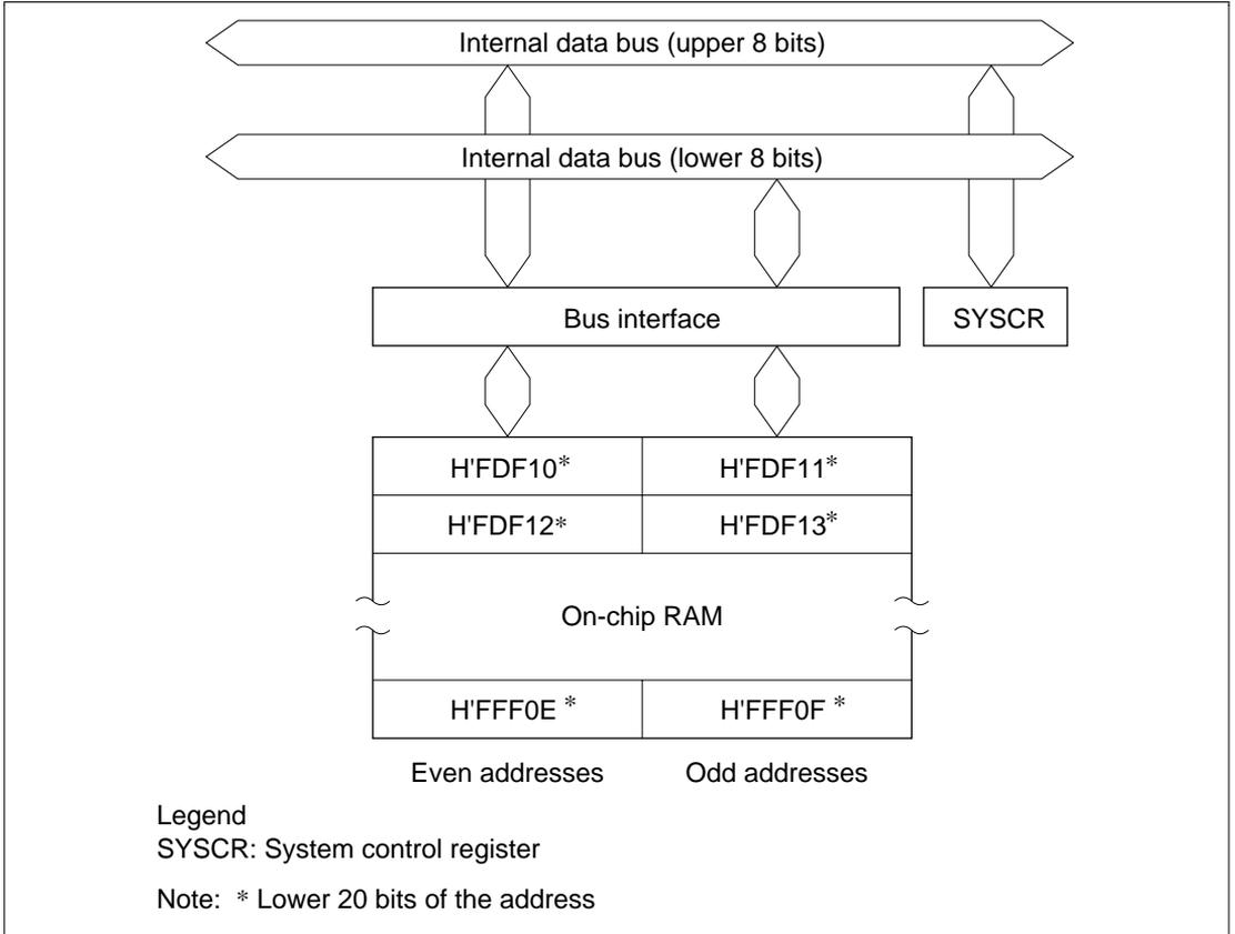
**Figure 14-1 RAM Block Diagram (H8/3022 in Modes 1, 5, 6 and 7)**
