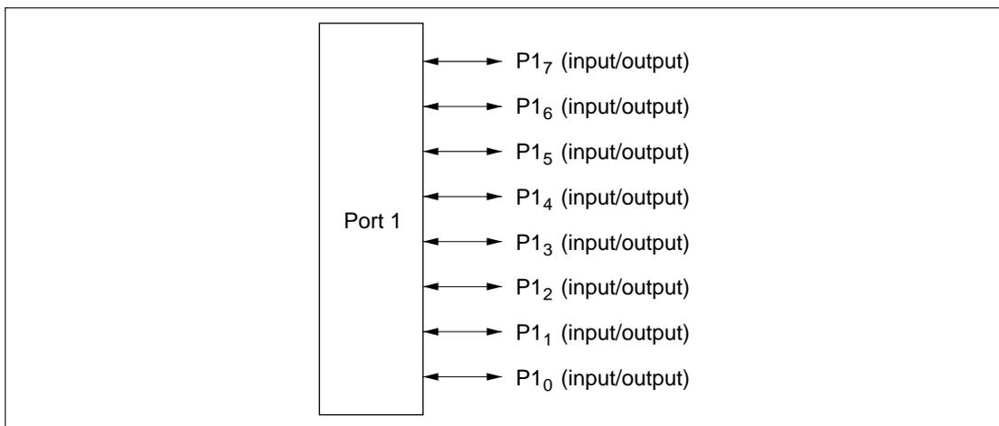
**Figure 7-4 Pin Functions in Mode 7 (Port 1)**
