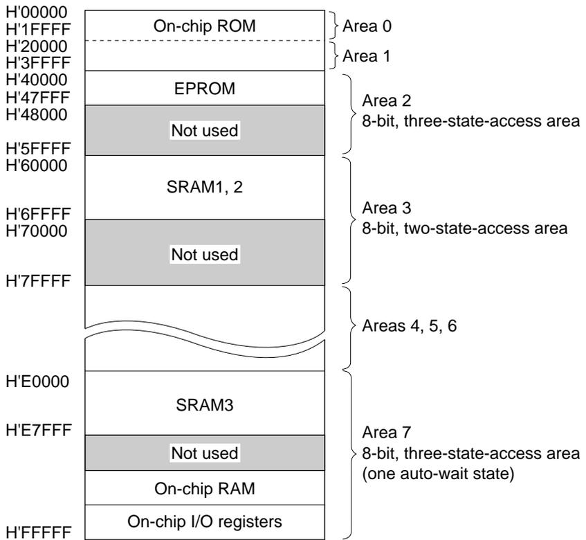
Note: The bus width and the number of access states of the on-chip memories and I/O registers are fixed; they cannot be changed by register setting.
