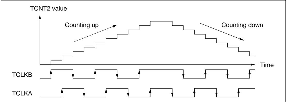
**Figure 8-44 Operation in Phase Counting Mode (Example)**
