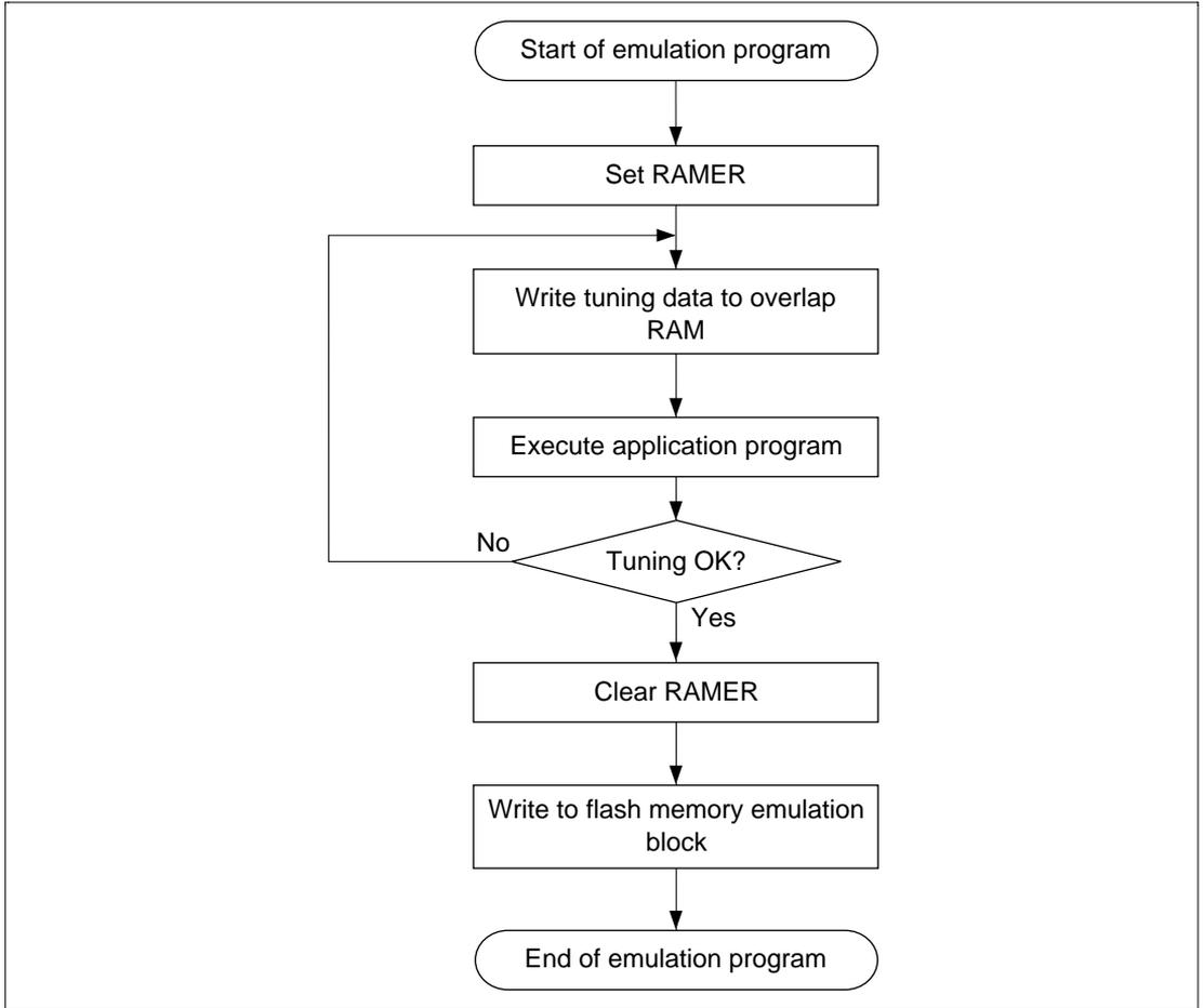
**Figure 15-14** Flowchart for Flash Memory Emulation in RAM
