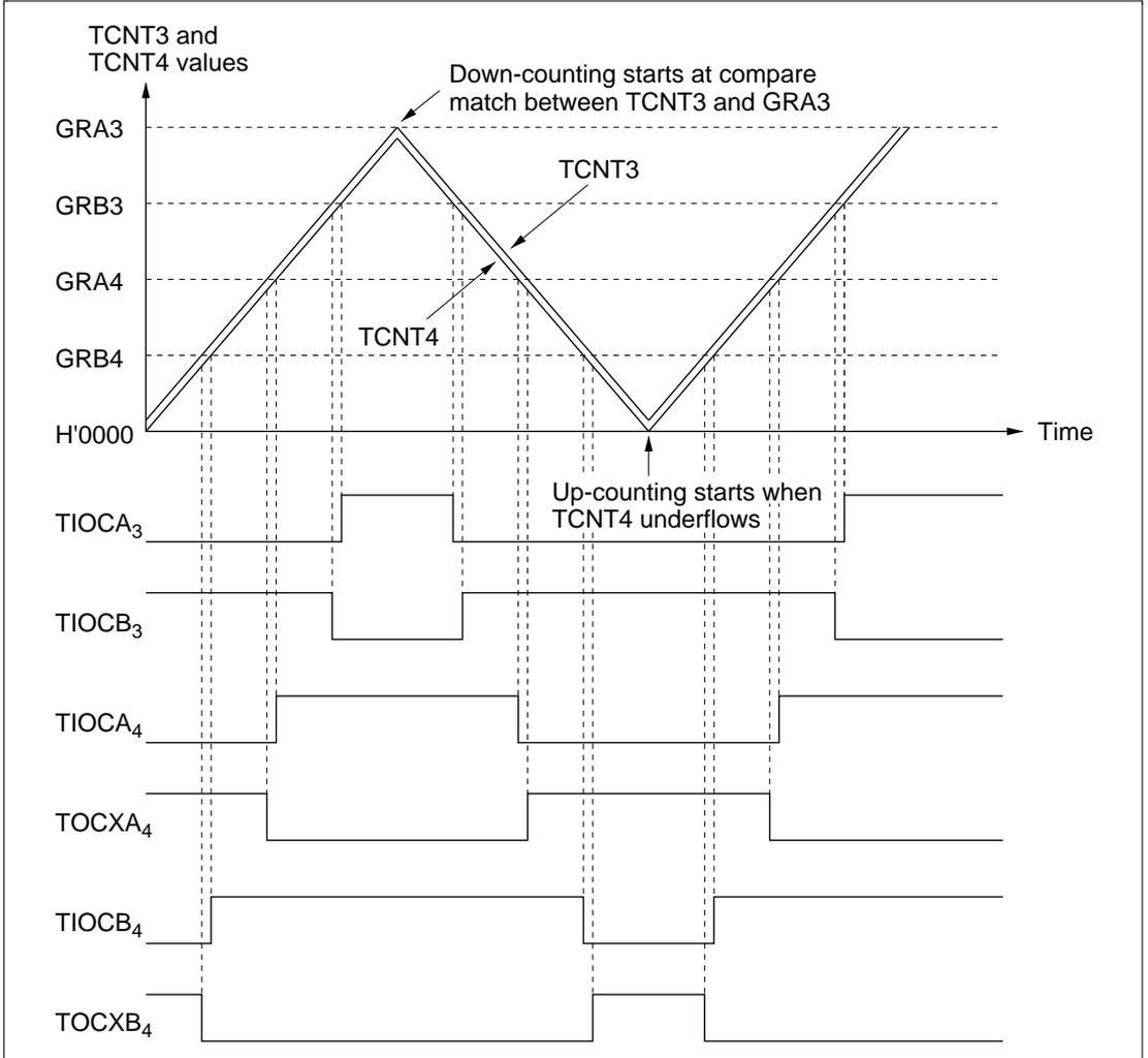
**Figure 8-35 Operation in Complementary PWM Mode (Example 1)**
