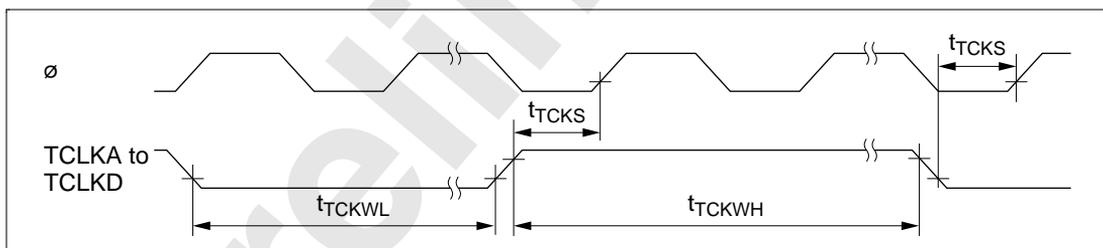
**Figure 18-16 ITU External Clock Input Timing**
