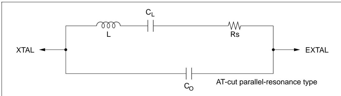
**Figure 16-3 Crystal Resonator Equivalent Circuit**
