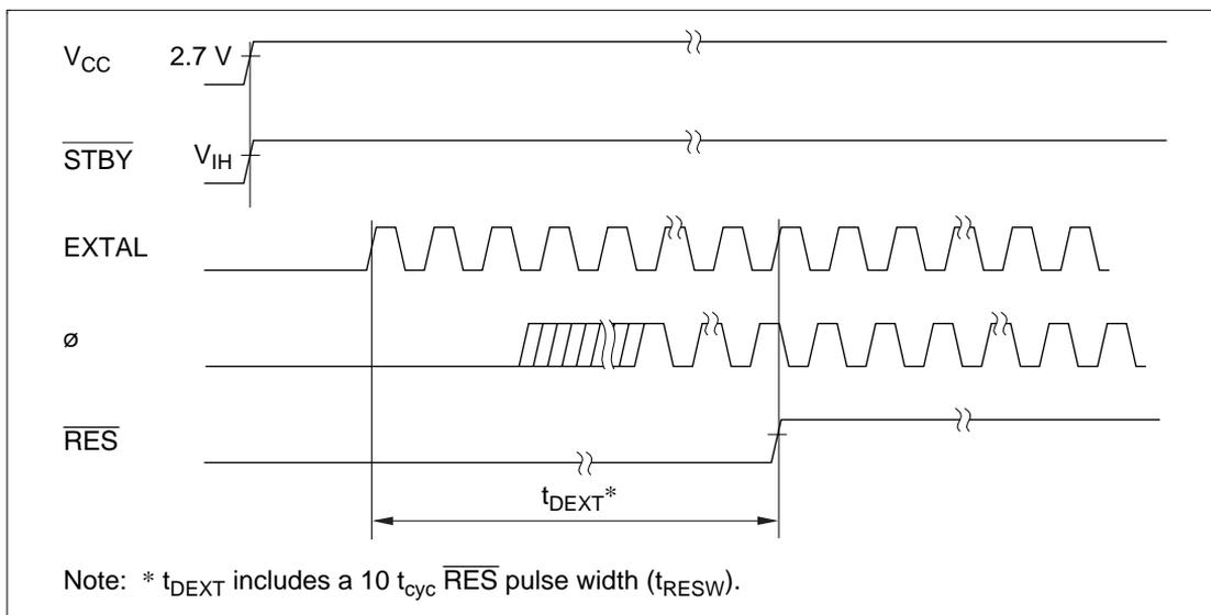
**Figure 16-7 External Clock Output Stabilization Delay Time**
