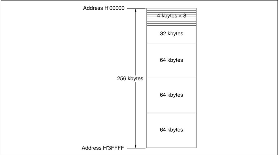
**Figure 15-5 Block Configuration**
