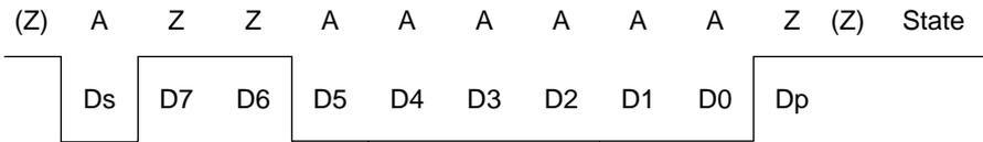
With the inverse convention type, the logic 1 level corresponds to state A and the logic 0 level to state Z, and transfer is performed in MSB-first order. The start character data above is H'3F.
