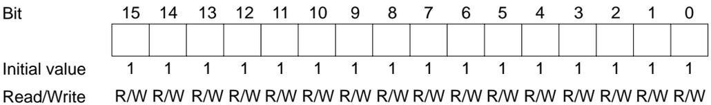
A buffer register is a 16-bit readable/writable register that is used when buffering is selected. Buffering can be selected independently by bits BFB4, BFA4, BFB3, and BFA3 in TFCR.
