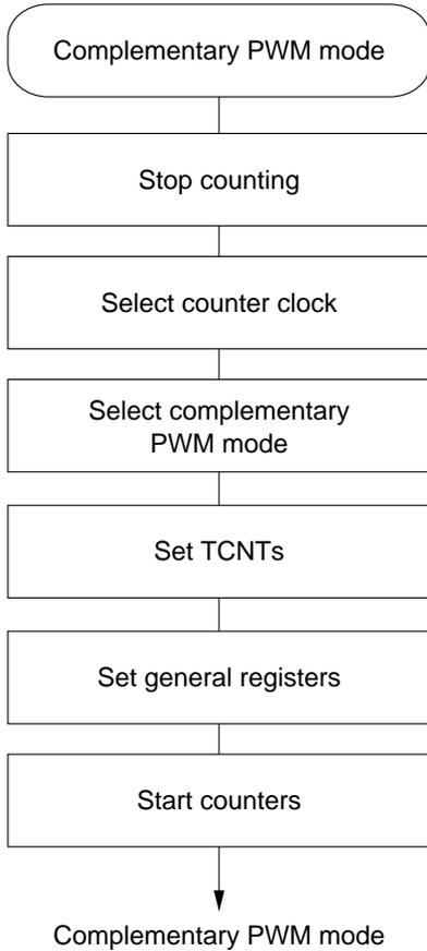
1. Clear bits STR3 and STR4 to 0 in TSTR to halt the timer counters. Complementary PWM mode must be set up while TCNT3 and TCNT4 are halted.
