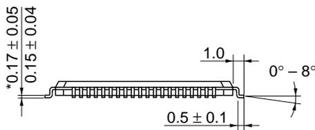
\*Dimension including the plating thickness
