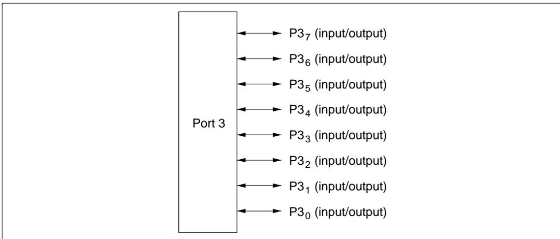
**Figure 7-11 Pin Functions in Mode 7 (Port 3)**
