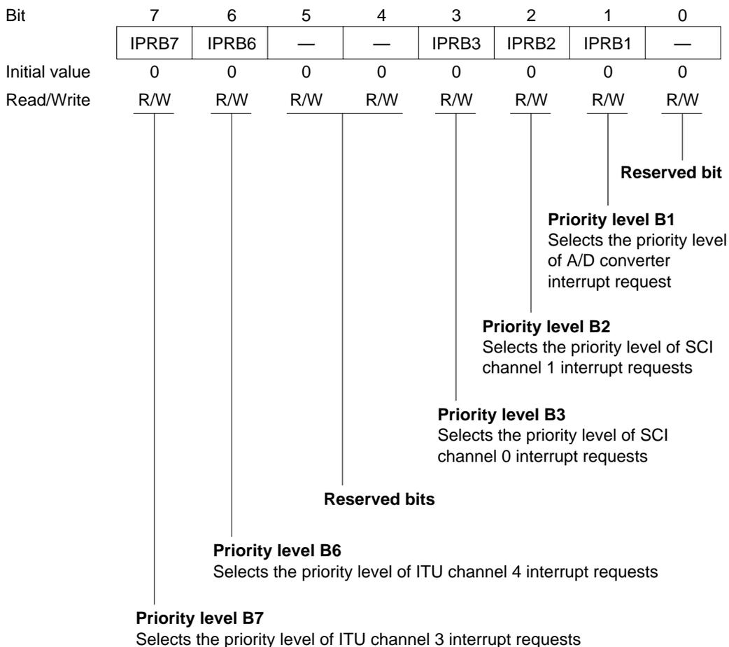
IPRB is initialized to H'00 by a reset and in hardware standby mode.
