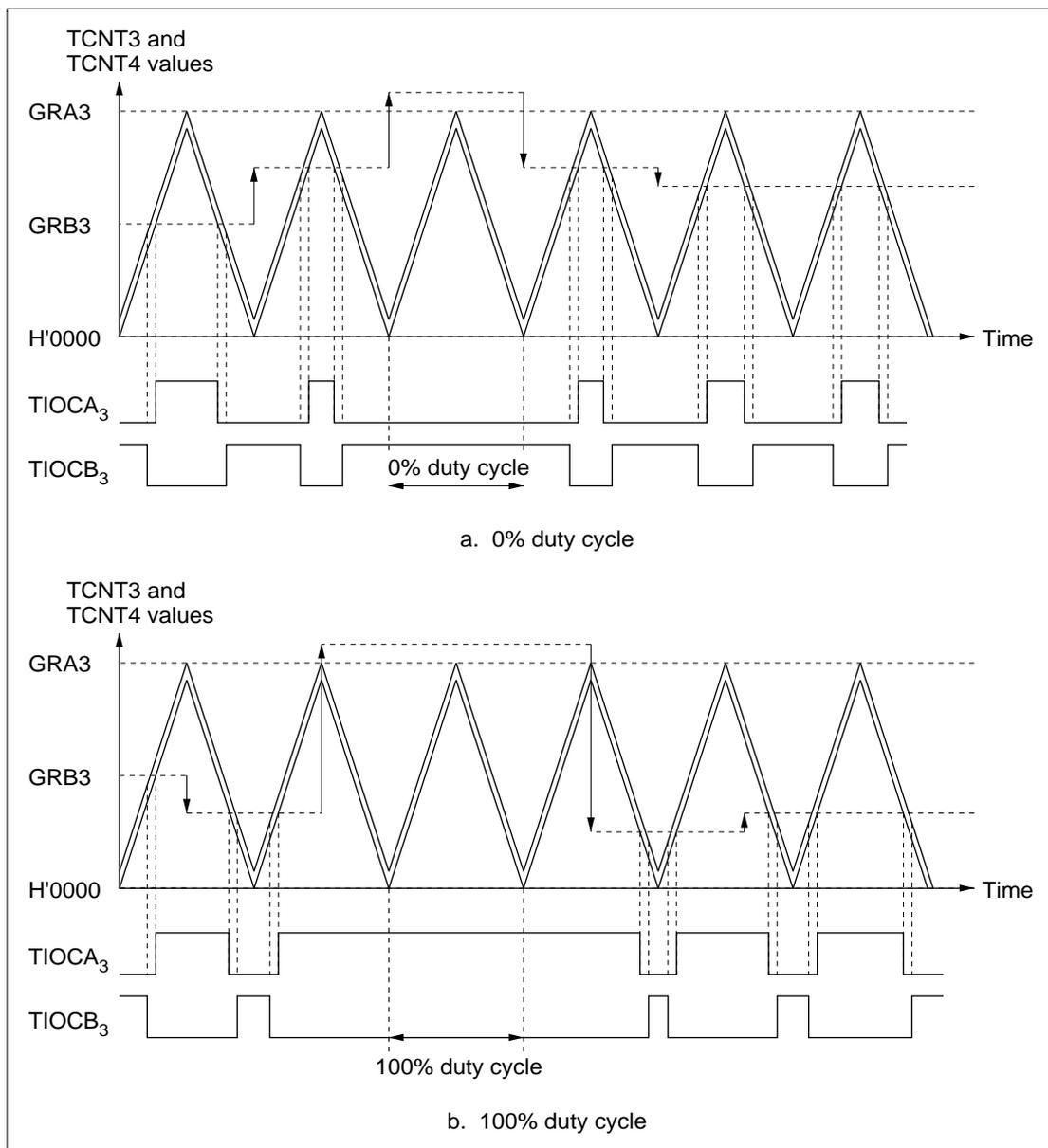
**Figure 8-36 Operation in Complementary PWM Mode (Example 2)**
