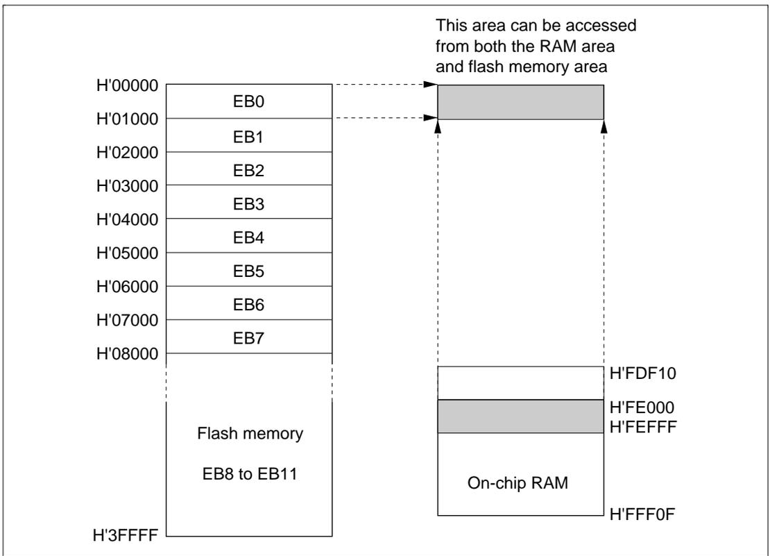
**Figure 15-15 Example of RAM Overlap Operation**
