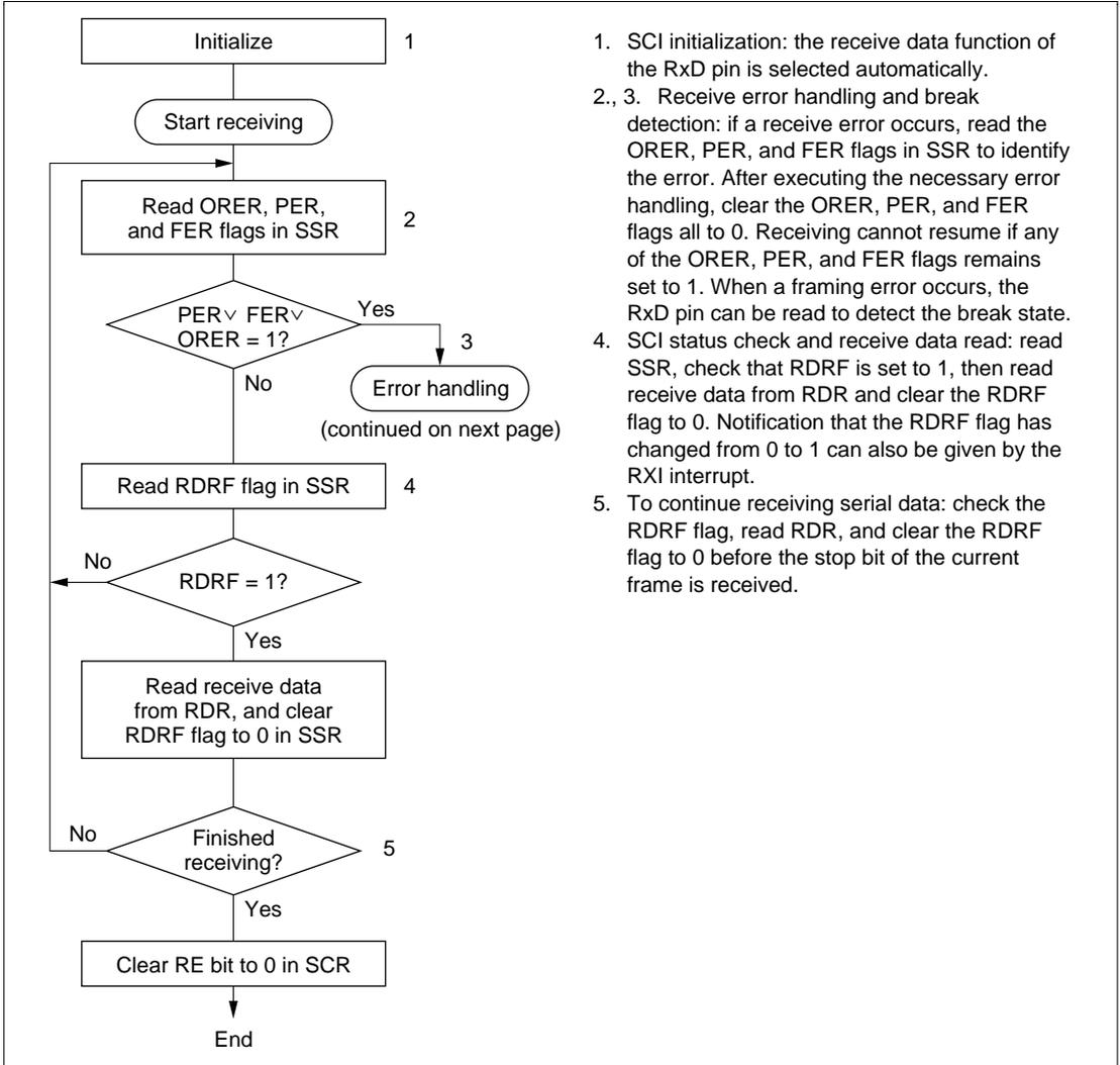
1. SCI initialization: the receive data function of the RxD pin is selected automatically.
