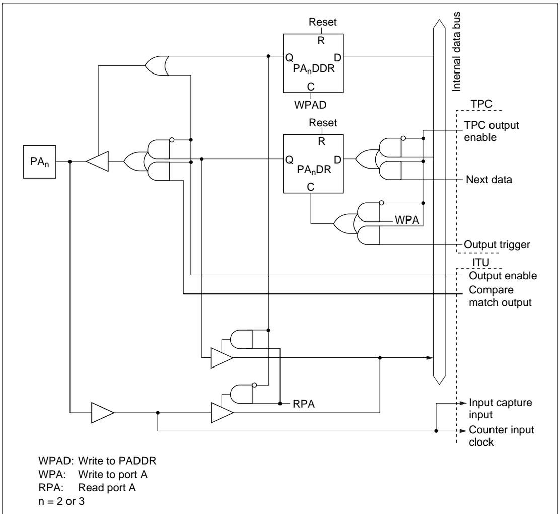
**Figure C-9 (b) Port A Block Diagram (Pins PA<sub>2</sub> and PA<sub>3</sub>)**
