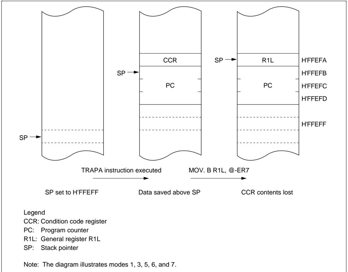
Figure 4-5 Operation when SP Value is Odd
