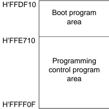
Note: The boot program area cannot be used until the programming control program transferred to RAM switches to the execution state. Note also that the boot program remains in this area in RAM even after control branches to the programming control program.
