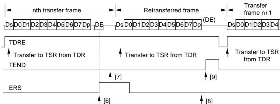
**Figure 12-9 Retransfer Operation in SCI Transmit Mode**
