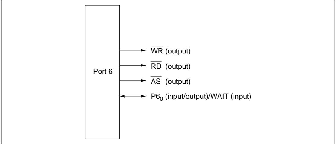
**Figure 7-17 Pin Functions in Modes 1, 3, 5, and 6 (Port 6)**
