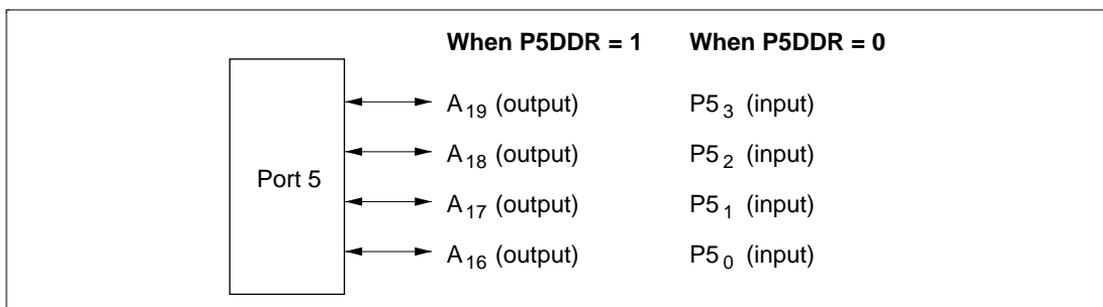
**Figure 7-14 Pin Functions in Modes 5 and 6 (Port 5)**
