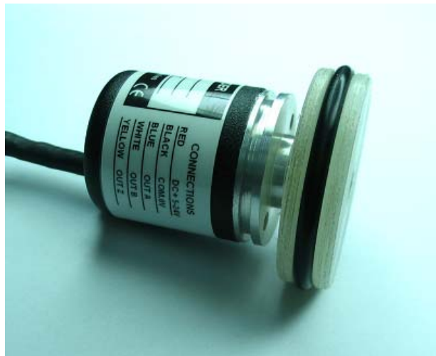
Rotary encoder connected to roller or wheel.
