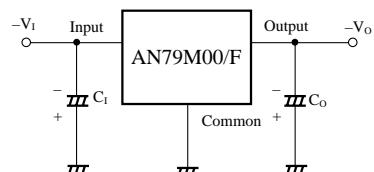
C<sub>I</sub> is connected when the input line is long. 2μF
