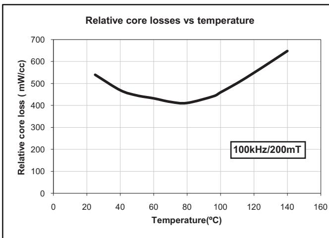
All measurements made on Toroid OD= 30mm, ID=20mm Ht=10mm.
