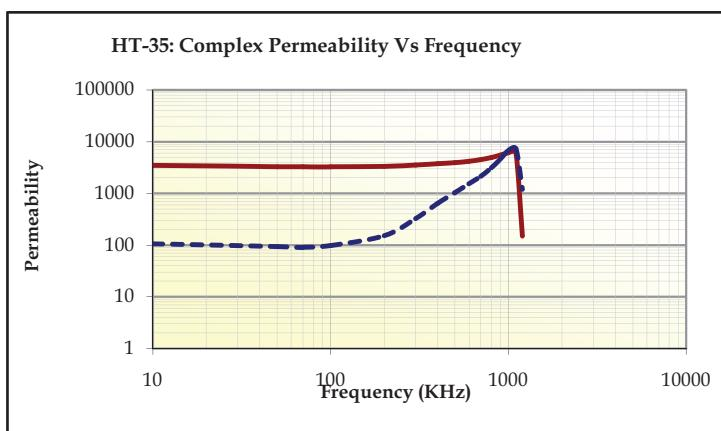
All measurements made on Toroid OD= 30mm, ID=20mm Ht=10mm.
