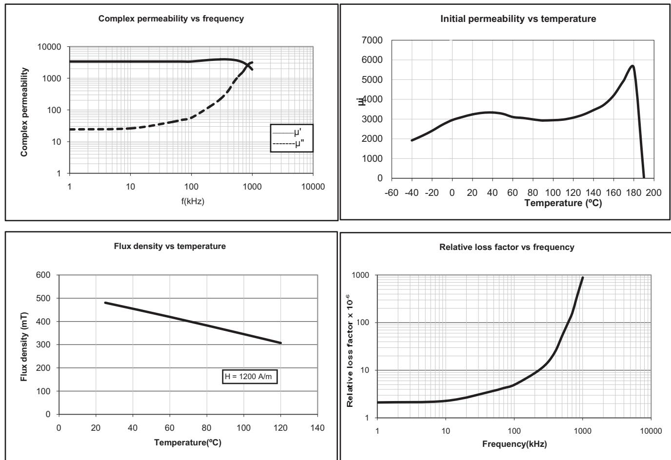
All measurements made on Toroid OD= 30mm, ID=20mm Ht=10mm.
