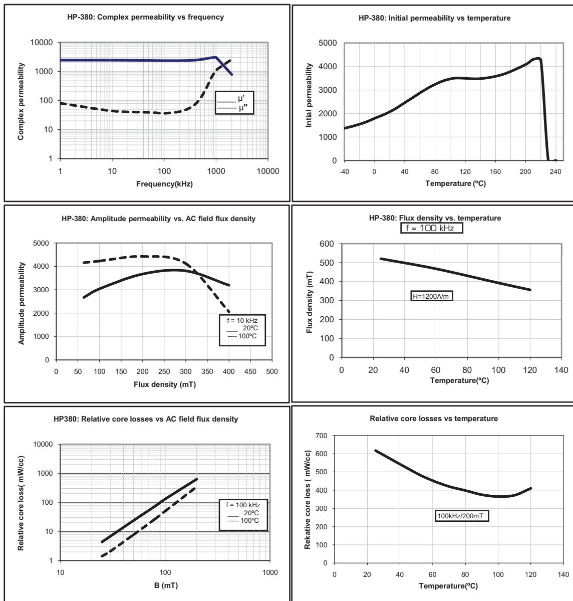
All measurements made on Toroid OD= 30mm, ID=20mm Ht=10mm.
