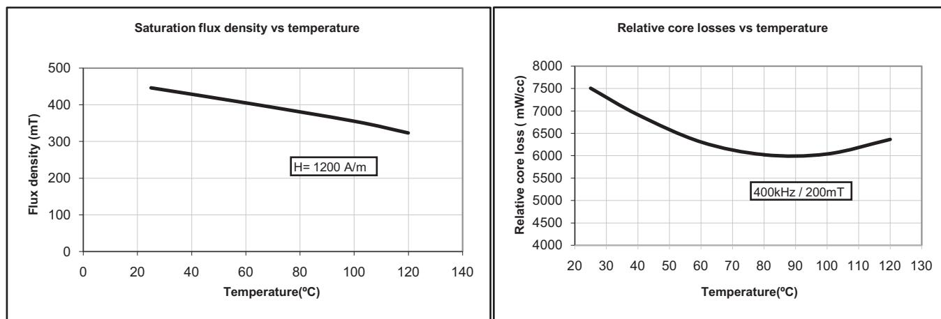
All measurements made on Toroid OD= 30mm, ID=20mm Ht=10mm.
