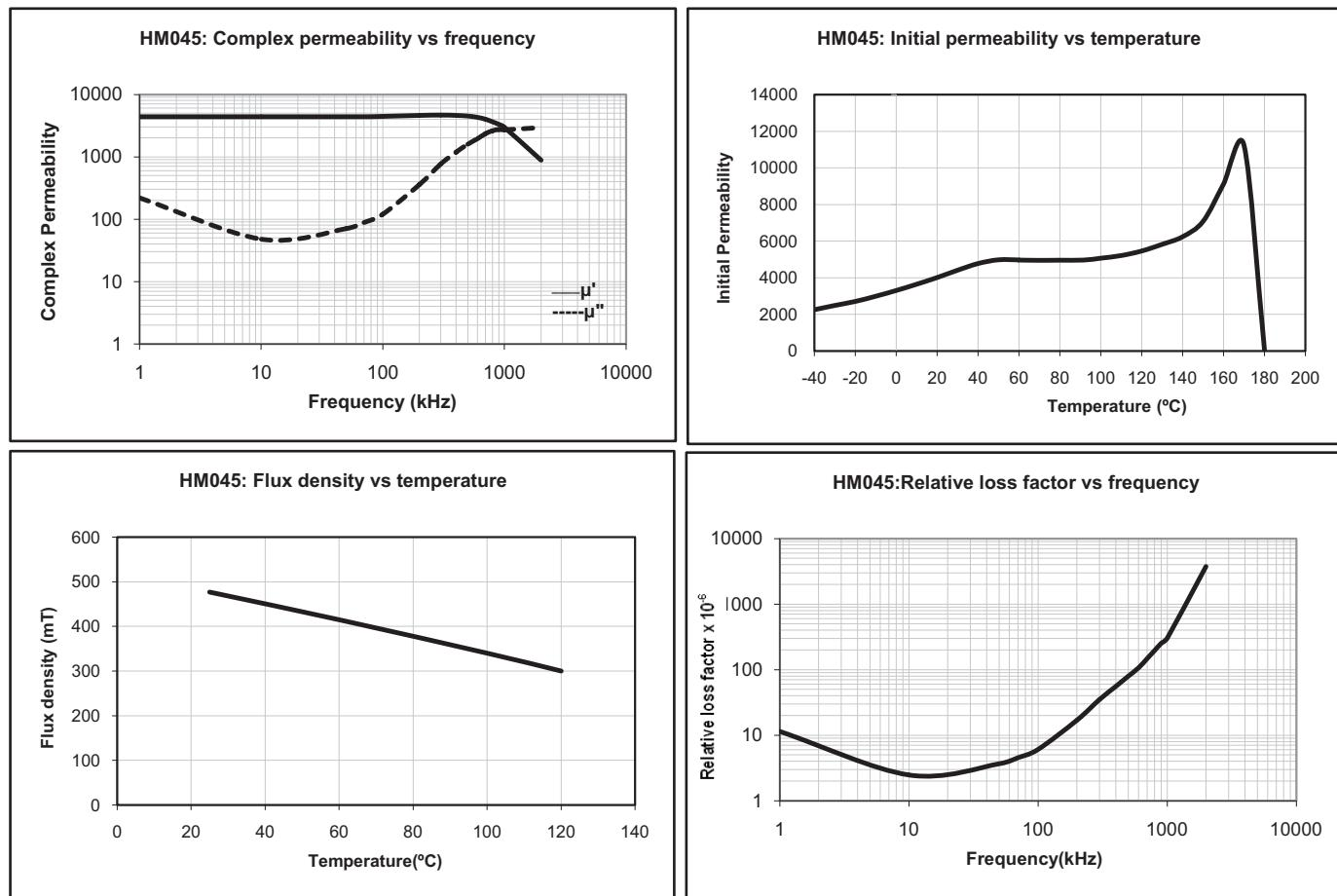
All measurements made on Toroid OD= 22mm, ID=14mm Ht=6mm.
