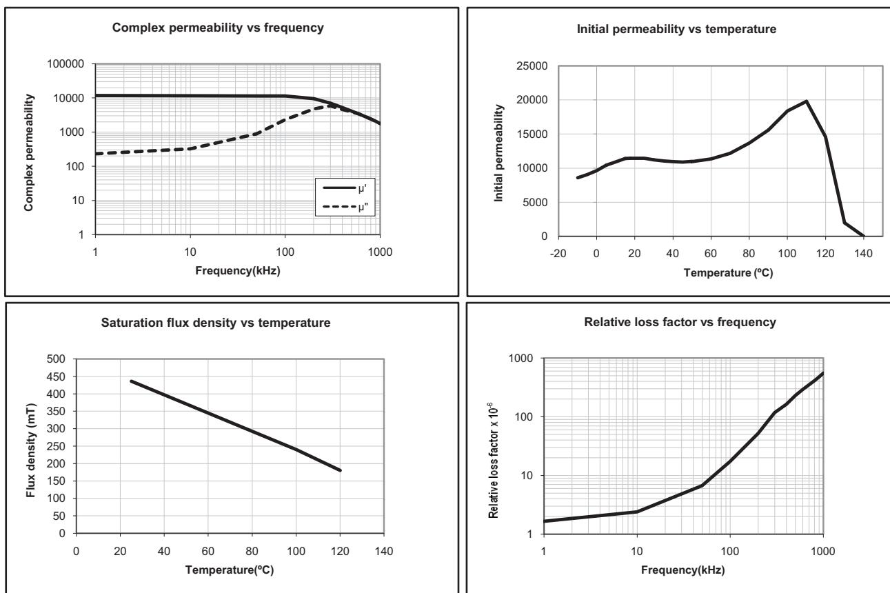
All measurements made on Toroid OD= 10mm, ID=06mm Ht=04mm
