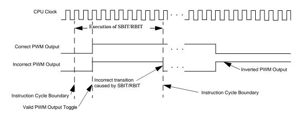
Workaround: The user should be aware of the state of Timers T2 and T3 before any SBIT or RBIT instructions are executed which operate on the PORTLD register.
