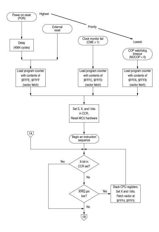
Figure 10-1 Processing flow out of reset (1 of 2)
