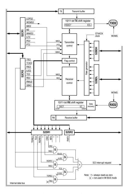
Figure 6-3 MI BUS block diagram
