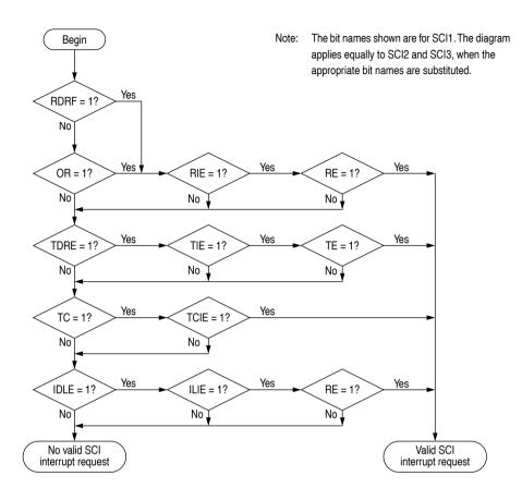
Figure 10-6 Interrupt source resolution within the SCI subsystem
