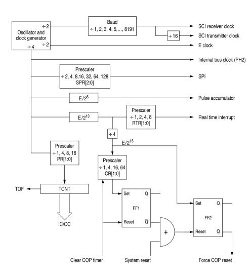
Figure 8-1 Timer clock divider chains
