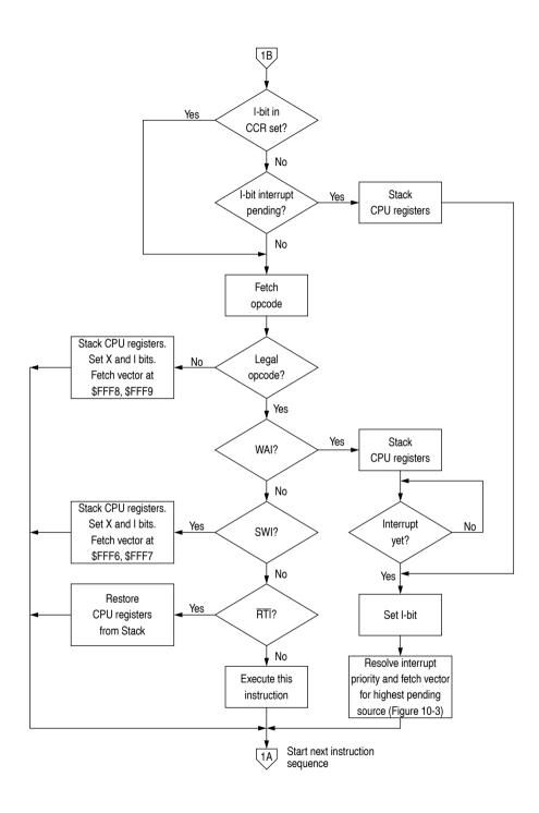
Figure 10-2 Processing flow out of reset (2 of 2)
