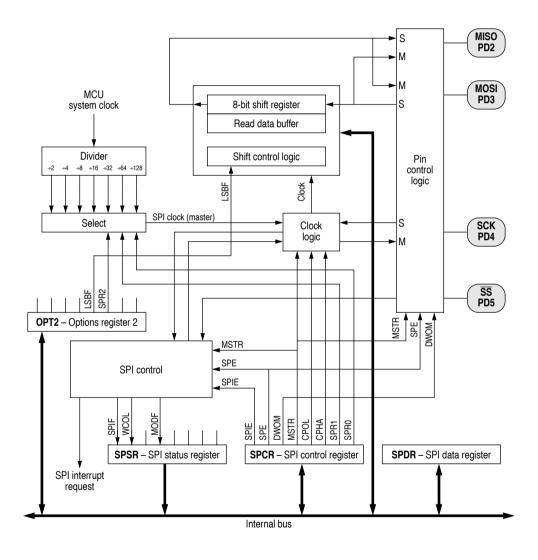
Figure 7-1 SPI block diagram
