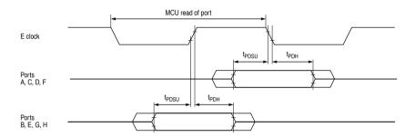
Figure 12-7 Port read timing diagram
