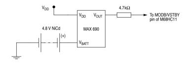
Figure 2-6 RAM stand-by connections
