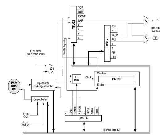
Figure 8-3 Pulse accumulator block diagram
