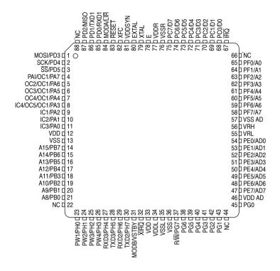
Figure 13-2 88-pin QFP pinout
