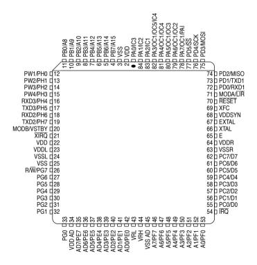
Figure 13-1 84-pin PLCC/CERQUAD pinout
