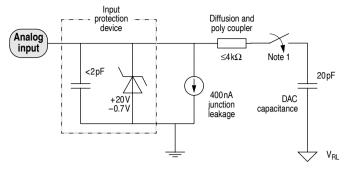
Note 1: The analog switch is closed only during the 12 cycle sample time Note 2: All component values are approximate
