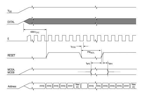
Figure 12-3 Reset timing
