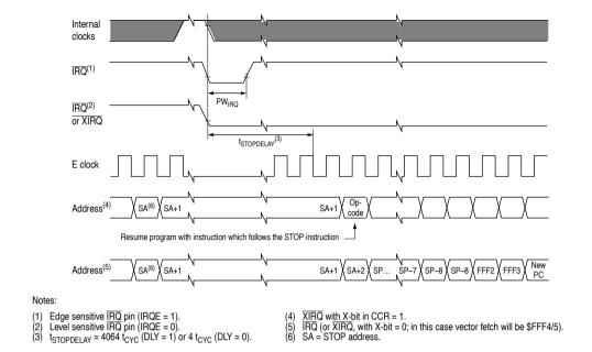
Figure 12-5 STOP recovery timing
