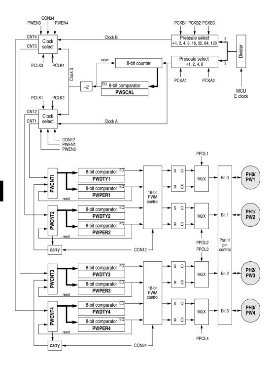
Figure 8-4 PWM timer block diagram
