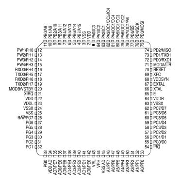
Figure 2-1 84-pin PLCC/CERQUAD pinout
