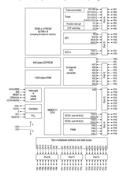
Figure 1-1 MC68HC11P2/MC68HC711P2 block diagram
