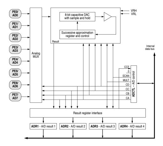
Figure 9-1 A/D converter block diagram
