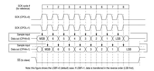
Figure 7-2 SPI transfer format
