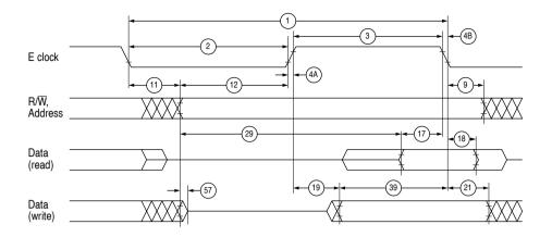
Figure 12-13 Expansion bus timing
