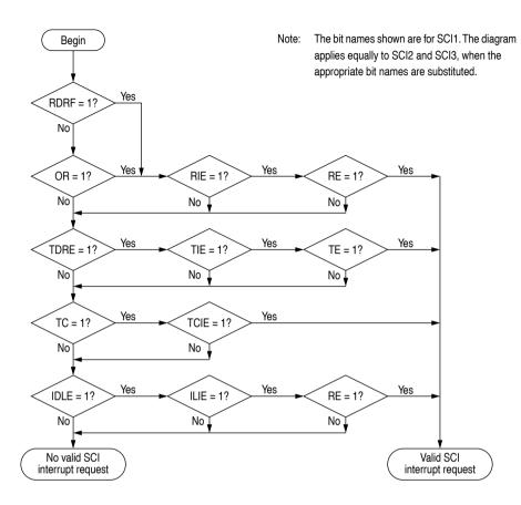
Figure 5-3 Interrupt source resolution within SCI
