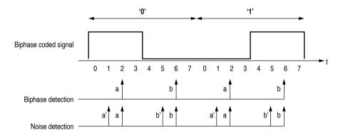
Figure 6-2 Biphase coding and error detection
