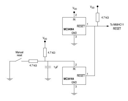
Figure 2-3 External reset circuitry
