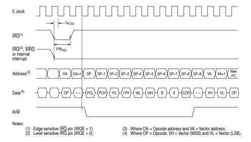
Figure 12-4 Interrupt timing
