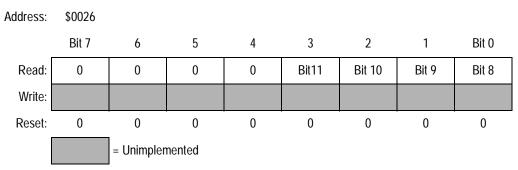
Figure 9-29. PWM Counter Register High (PCNTH)
