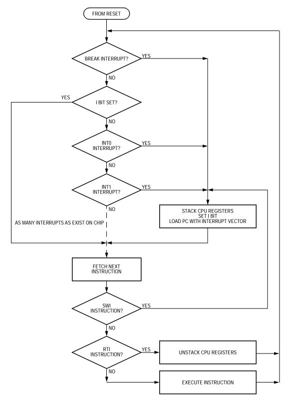
Figure 7-9. Interrupt Processing
