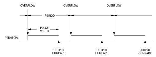
Figure 12-3. PWM Period and Pulse Width
