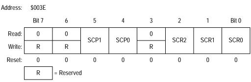
Figure 13-14. SCI Baud Rate Register (SCBR)
