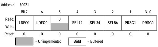
Figure 9-36. PWM Control Register 2 (PCTL2)
