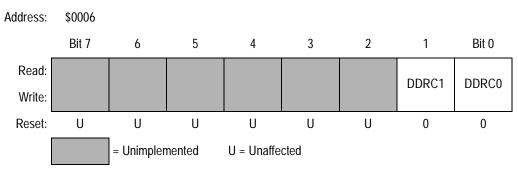
Figure 14-9. Data Direction Register C (DDRC)
