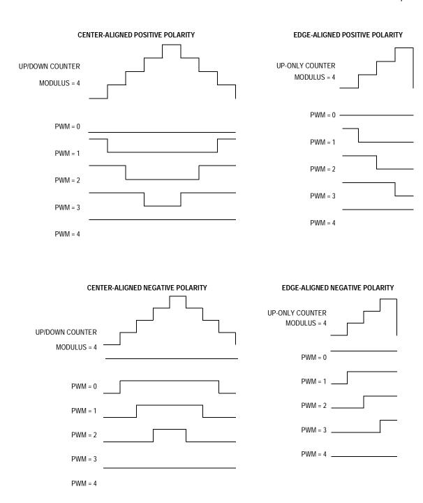
Figure 9-17. PWM Polarity
