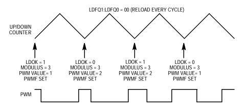
Figure 9-7. Center-Aligned PWM Value Loading
