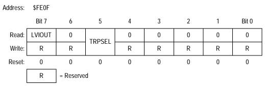
Figure 17-3. LVI Status and Control Register (LVISCR)
