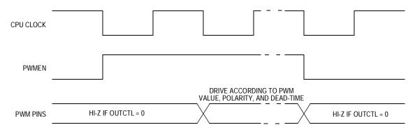
Figure 9-28. PWMEN and PWM Pins
