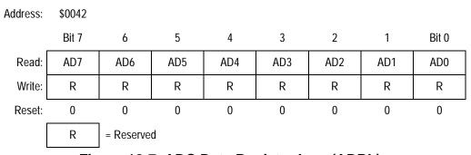
Figure 18-7. ADC Data Register Low (ADRL)
