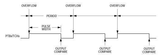
Figure 11-3. PWM Period and Pulse Width
