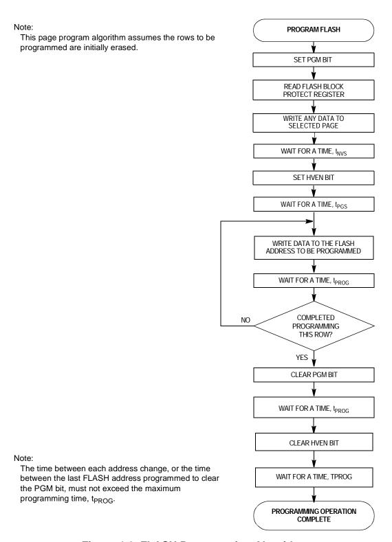
Figure 4-2. FLASH Programming Algorithm
