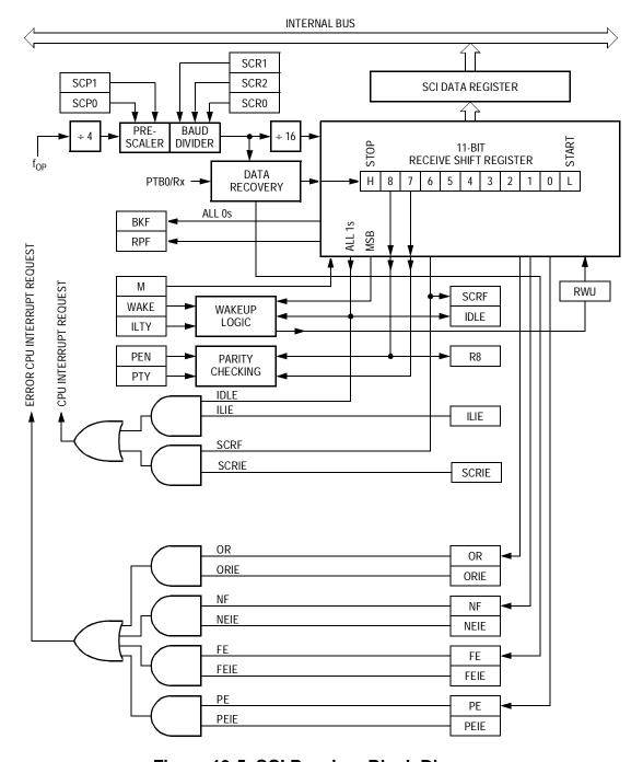
Figure 13-5. SCI Receiver Block Diagram
