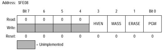
Figure 4-1. FLASH Control Register (FLCR)
