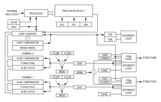
Figure 12-1. TIMB Block Diagram
