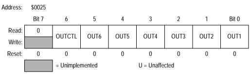
Figure 9-42. PWM Output Control Register (PWMOUT)
