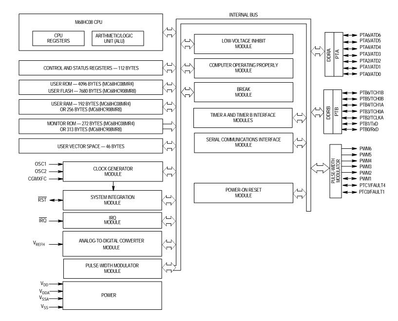
Figure 1-1. MCU Block Diagram
