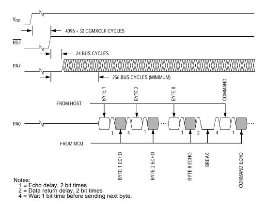
Figure 10-6. Monitor Mode Entry Timing
