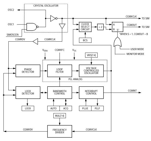
Figure 8-1. CGM Block Diagram
