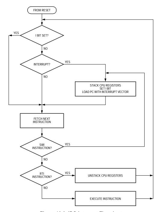
Figure 16-3. IRQ Interrupt Flowchart
