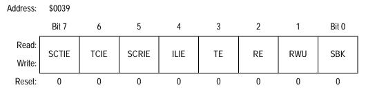
Figure 13-8. SCI Control Register 2 (SCC2)
