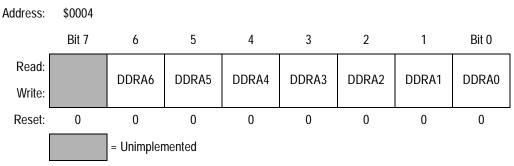
Figure 14-3. Data Direction Register A (DDRA)
