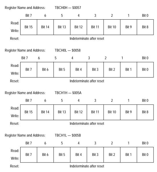
Figure 12-9. TIMB Channel Registers (TBCH0H/L-TBCH1H/L)
