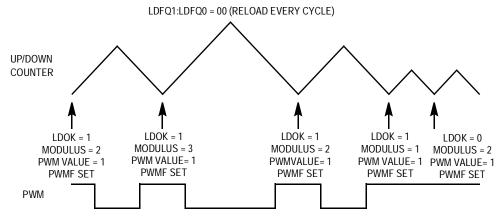
Figure 9-8. Center-Aligned Loading of Modulus
