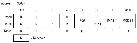
Figure 16-4. IRQ Status and Control Register (ISCR)
