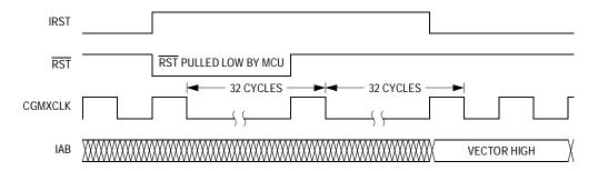
Figure 7-5. Internal Reset Timing
