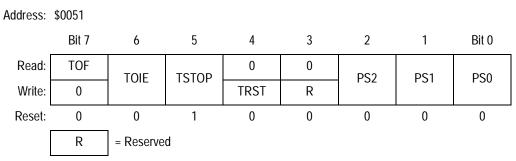
Figure 12-4. TIMB Status and Control Register (TBSC)
