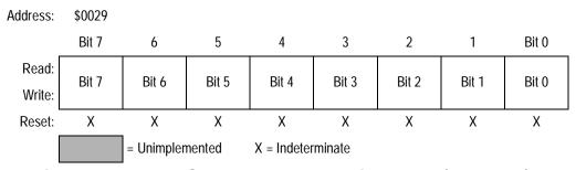
Figure 9-32. PWM Counter Modulo Register Low (PDMODL)
