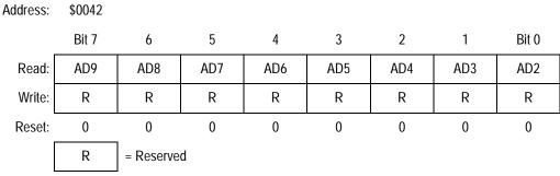
Figure 18-8. ADC Data Register Low (ADRL) 8-Bit Mode
