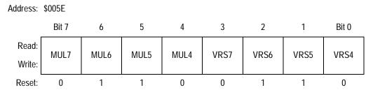
Figure 8-7. PLL Programming Register (PPG)
