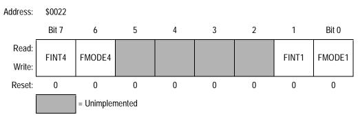
Figure 9-39. Fault Control Register (FCR)
