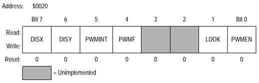
Figure 9-35. PWM Control Register 1 (PCTL1)
