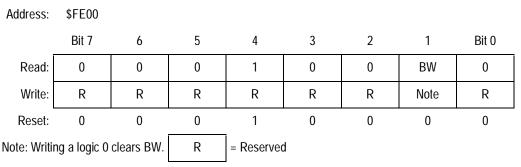
Figure 20-6. SIM Break Status Register (SBSR)
