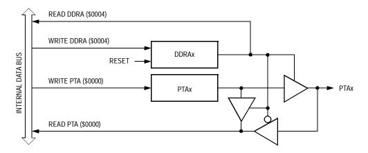
Figure 14-4. Port A I/O Circuit
