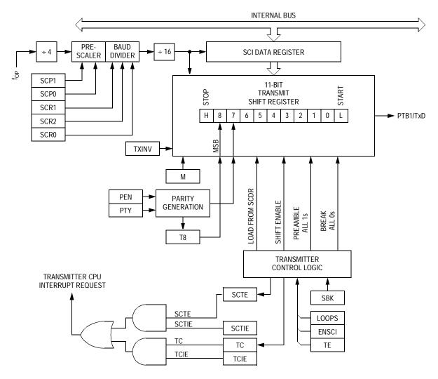
Figure 13-4. SCI Transmitter
