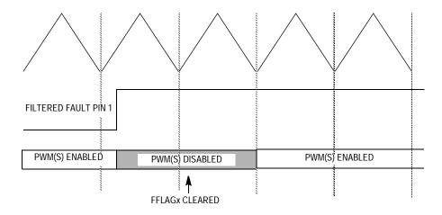
Figure 9-25. PWM Disabling in Manual Mode (Example 1)
