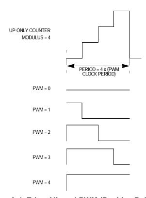
Figure 9-4. Edge-Aligned PWM (Positive Polarity)
