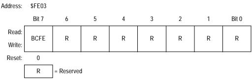
Figure 20-8. SIM Break Flag Control Register (SBFCR)
