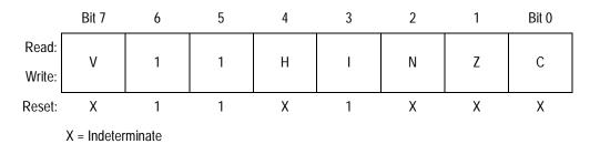
Figure 6-6. Condition Code Register (CCR)
