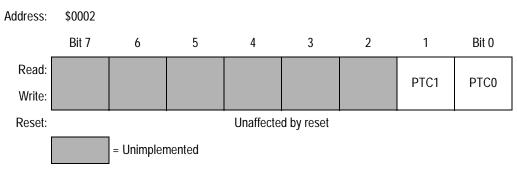
Figure 14-8. Port C Data Register (PTC)
