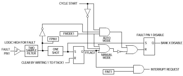
The example is of fault pin 1.
