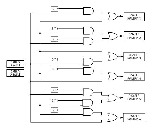
Figure 9-23. PWM Disabling Decode Scheme
