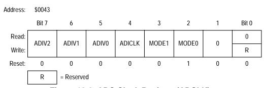
Figure 18-9. ADC Clock Register (ADCLK)
