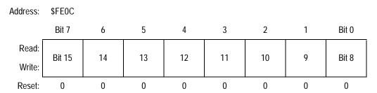
Figure 20-4. Break Address Register High (BRKH)
