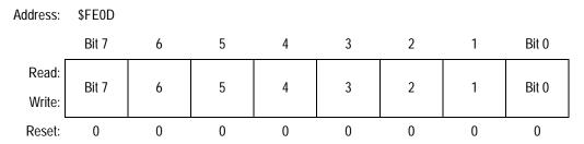
Figure 20-5. Break Address Register Low (BRKL)
