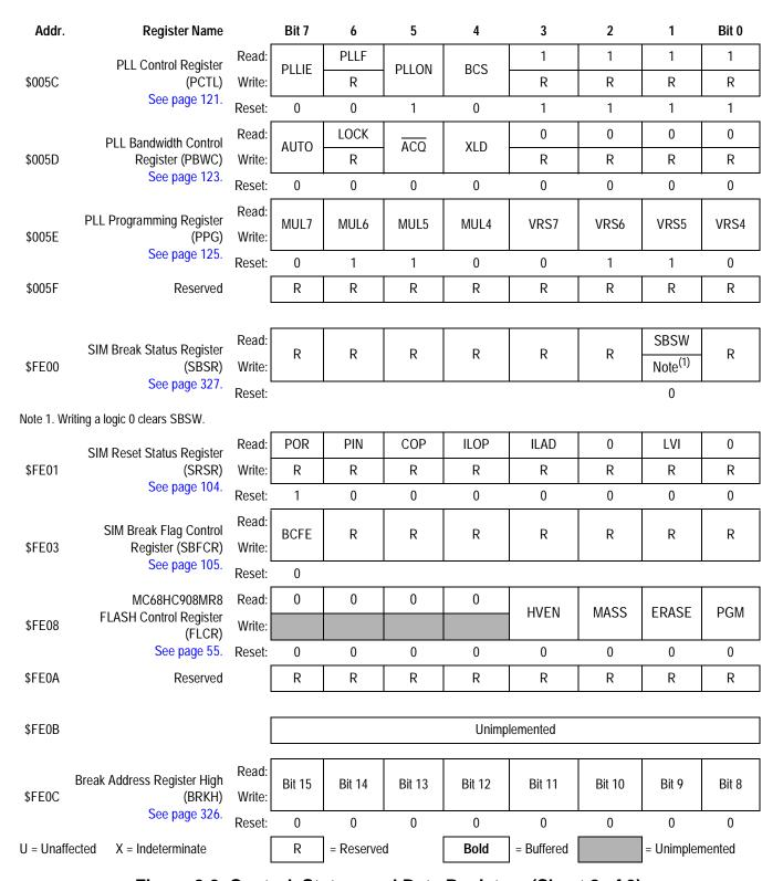
Figure 2-2. Control, Status, and Data Registers (Sheet 8 of 9)
