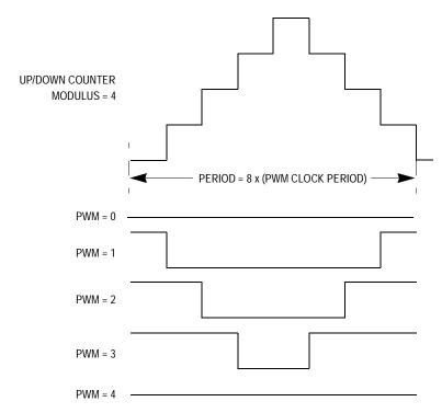
Figure 9-3. Center-Aligned PWM (Positive Polarity)
