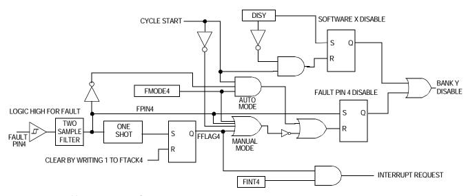
The example is of fault pin 4 with DISY.
