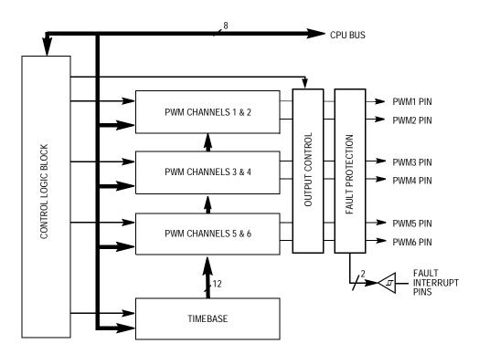
Figure 9-1. PWM Module Block Diagram
