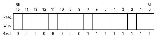
Figure 6-4. Stack Pointer (SP)
