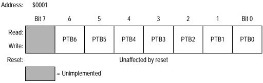
Figure 14-5. Port B Data Register (PTB)
