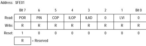
Figure 7-16. SIM Reset Status Register (SRSR)
