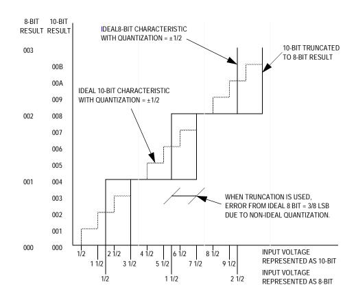
Figure 18-2. 8-Bit Truncation Mode Error
