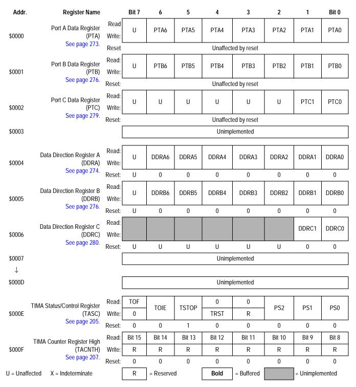
Figure 2-2. Control, Status, and Data Registers (Sheet 1 of 9)
