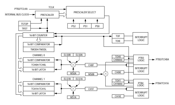
Figure 11-1. TIMA Block Diagram
