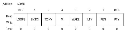
Figure 13-7. SCI Control Register 1 (SCC1)
