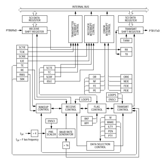
Figure 13-1. SCI Module Block Diagram
