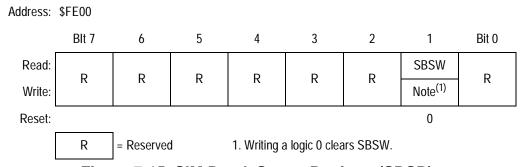
Figure 7-15. SIM Break Status Register (SBSR)
