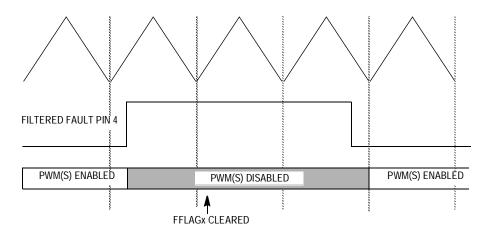
Figure 9-26. PWM Disabling in Manual Mode (Example 2)
