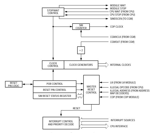
Figure 7-1. SIM Block Diagram
