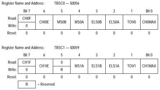
Figure 12-7. TIMB Channel Status and Control Registers (TBSC0–TBSC1)
