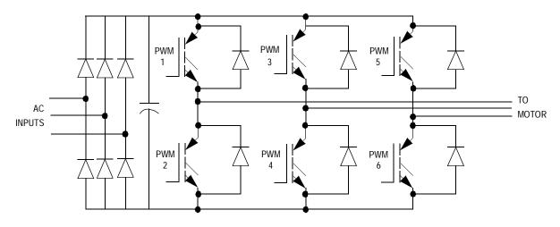
Figure 9-12. Typical AC Motor Drive
