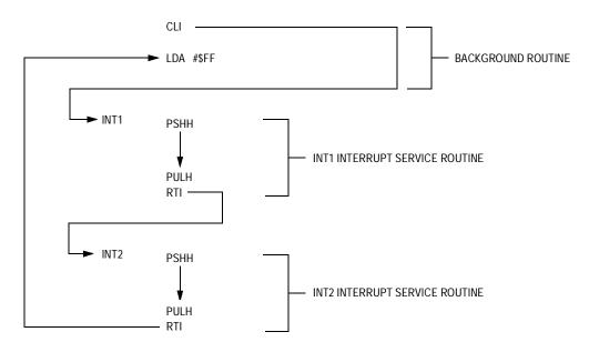
Figure 7-11. Interrupt Recognition Example
