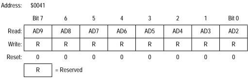
Figure 18-4. ADC Data Register High (ADRH)
