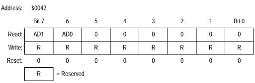
Figure 18-6. ADC Data Register Low (ADRL)
