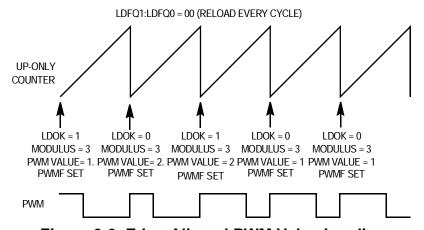
Figure 9-9. Edge-Aligned PWM Value Loading
