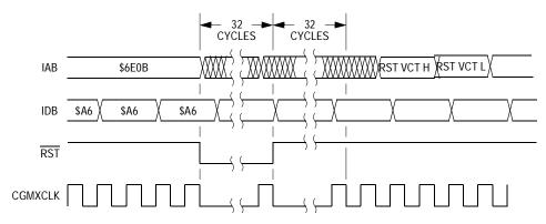
Figure 7-14. Wait Recovery from Internal Reset
