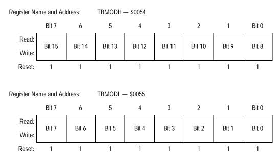
Figure 12-6. TIMB Counter Modulo Registers (TMODH and TMODL)
