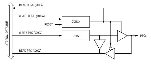
Figure 14-10. Port C I/O Circuit
