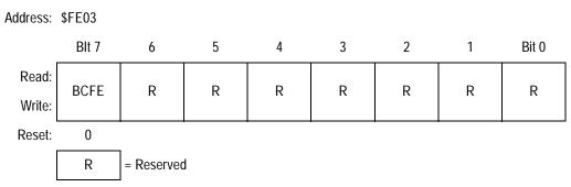
Figure 7-17. SIM Break Flag Control Register (SBFCR)
