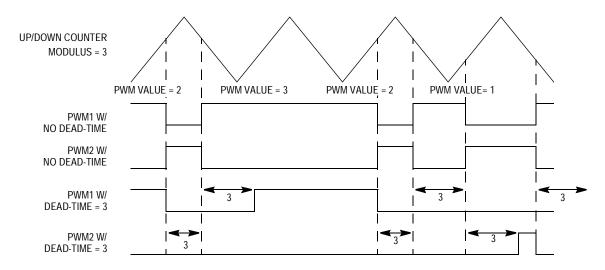
Figure 9-16. Dead-Time and Small Pulse Widths
