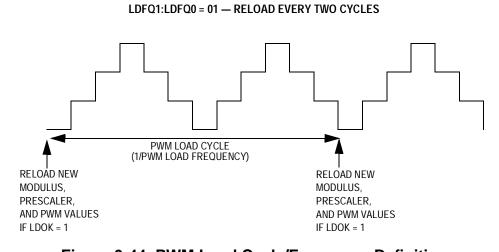
Figure 9-44. PWM Load Cycle/Frequency Definition
