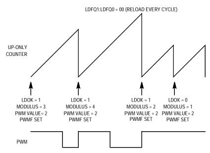
Figure 9-10. Edge-Aligned Modulus Loading
