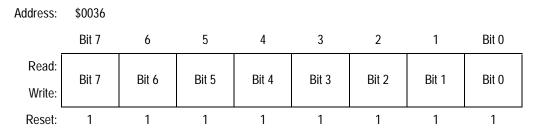
Figure 9-37. Dead-Time Write-Once Register (DEADTM)
