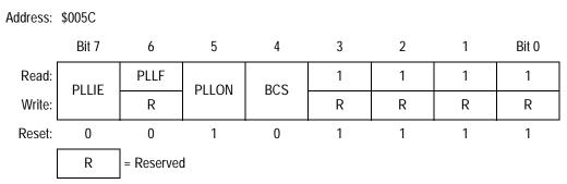
Figure 8-5. PLL Control Register (PCTL)
