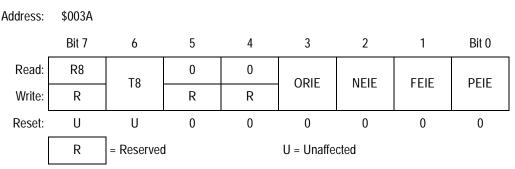
Figure 13-9. SCI Control Register 3 (SCC3)
