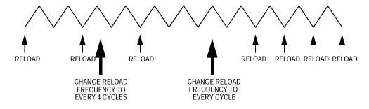
Figure 9-5. Reload Frequency Change
