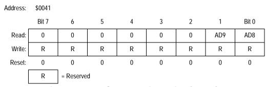
Figure 18-5. ADC Data Register High (ADRH)
