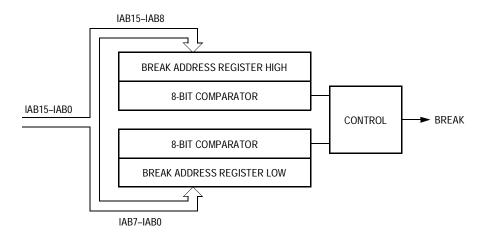
Figure 20-1. Break Module Block Diagram
