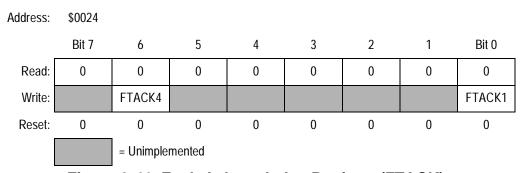
Figure 9-41. Fault Acknowledge Register (FTACK)
