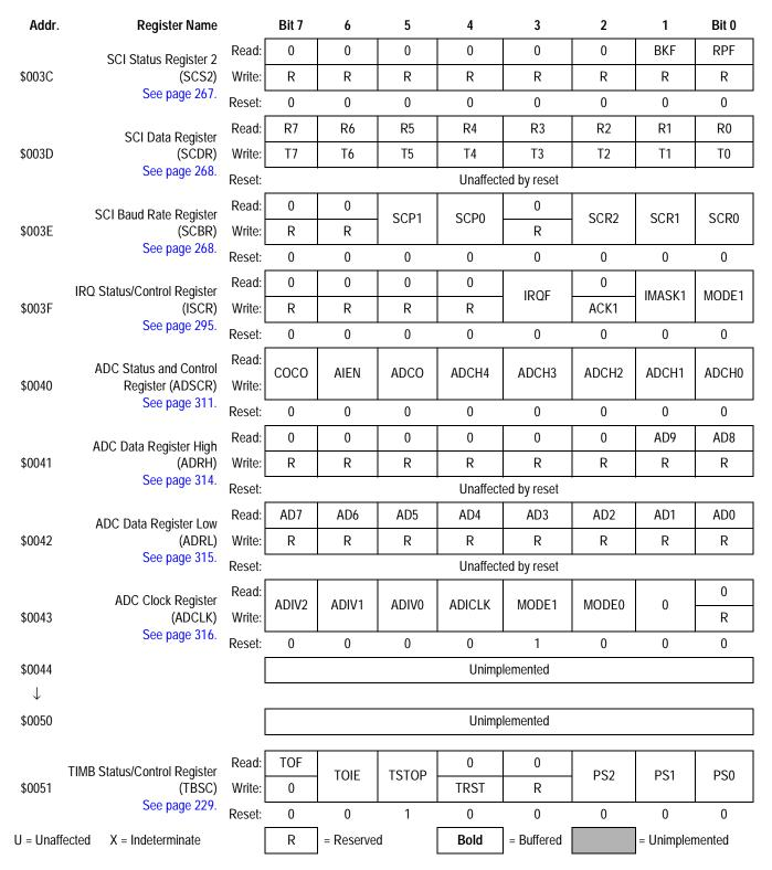
Figure 2-2. Control, Status, and Data Registers (Sheet 6 of 9)
