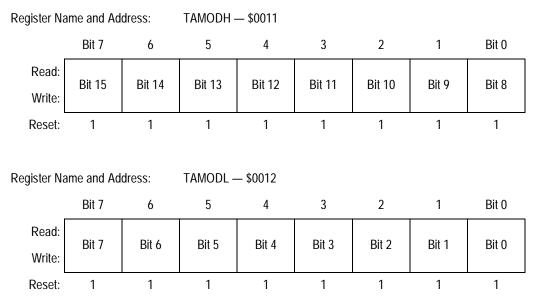
Figure 11-6. TIMA Counter Modulo Registers (TMODH and TMODL)
