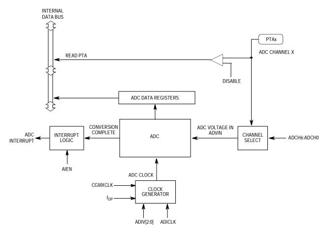
Figure 18-1. ADC Block Diagram
