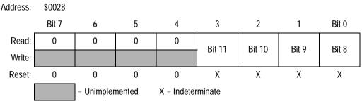
Figure 9-31. PWM Counter Modulo Register High (PDMODH)
