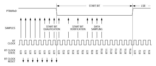
Figure 13-6. Receiver Data Sampling
