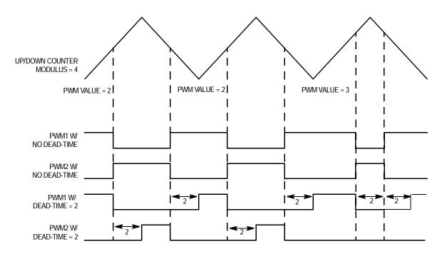
Figure 9-14. Effects of Dead-Time Insertion
