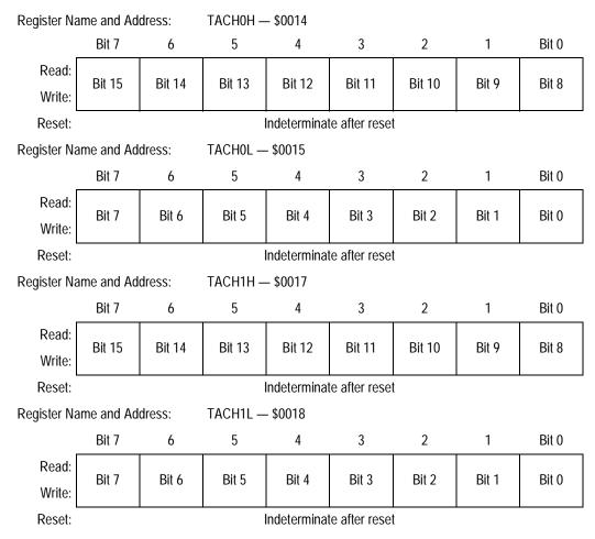
Figure 11-9. TIMA Channel Registers (TACH0H/L-TACH1H/L)
