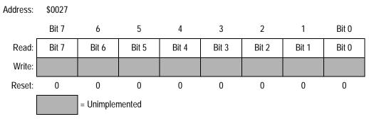
Figure 9-30. PWM Counter Register Low (PCNTH)
