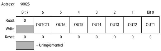
Figure 9-18. PWM Output Control Register (PWMOUT)
