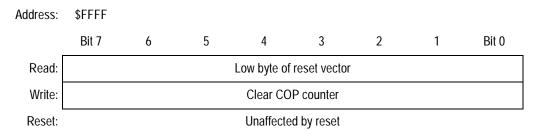
Figure 15-3. COP Control Register (COPCTL)
