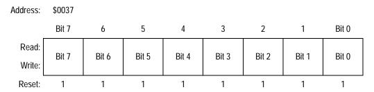
Figure 9-38. PWM Disable Mapping Write-Once Register (DISMAP)
