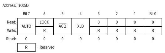
Figure 8-6. PLL Bandwidth Control Register (PBWC)
