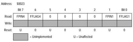
Figure 9-40. Fault Status Register (FSR)
