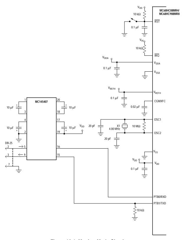
Figure 10-1. Monitor Mode Circuit
