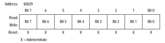
Figure 9-35. PWM Counter Modulo Register Low (PMODL)
