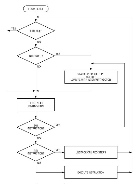
Figure 17-3. IRQ Interrupt Flowchart
