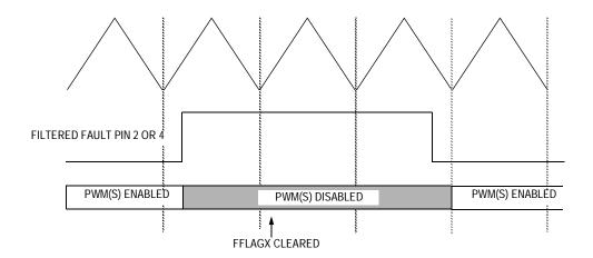
Figure 9-29. PWM Disabling in Manual Mode (Example 2)
