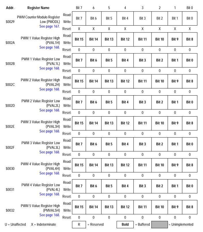
Figure 2-2. Control, Status, and Data Registers Summary (Sheet 5 of 10)
