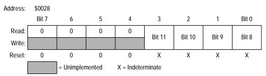
Figure 9-34. PWM Counter Modulo Register High (PMODH)
