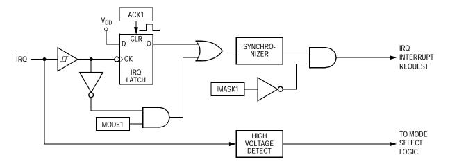
Figure 17-1. IRQ Module Block Diagram
