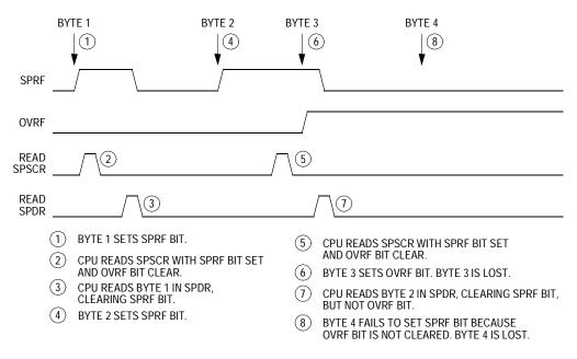
Figure 13-8. Missed Read of Overflow Condition
