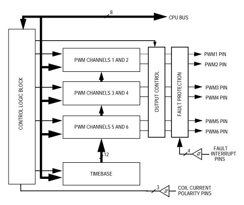
Figure 9-1. PWM Module Block Diagram
