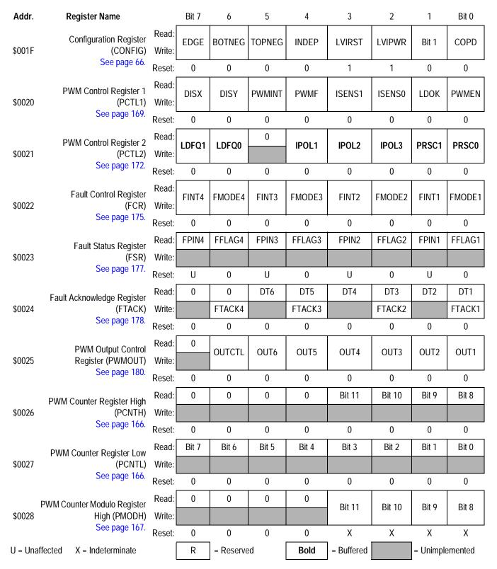
Figure 2-2. Control, Status, and Data Registers Summary (Sheet 4 of 10)
