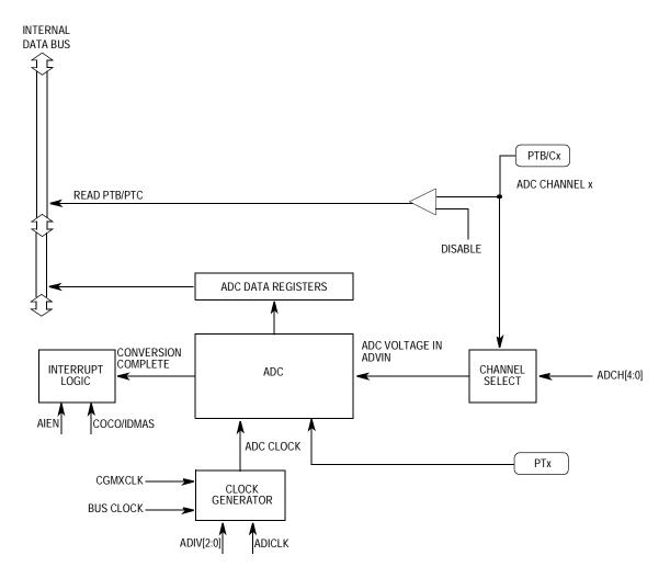
Figure 19-1. ADC Block Diagram
