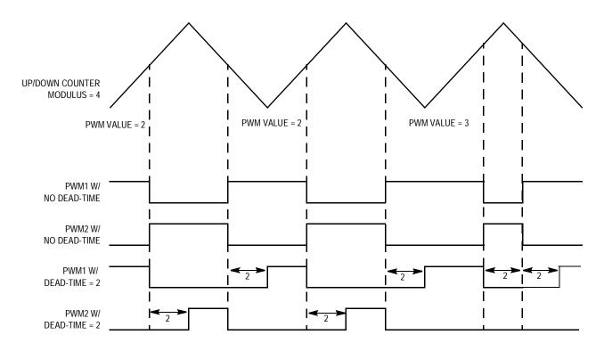
Figure 9-14. Effects of Dead-Time Insertion
