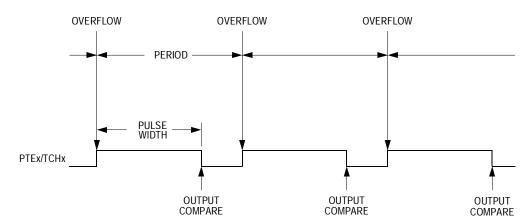
Figure 12-3. PWM Period and Pulse Width
