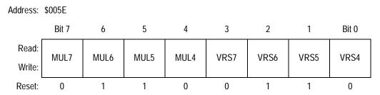
Figure 8-7. PLL Programming Register (PPG)
