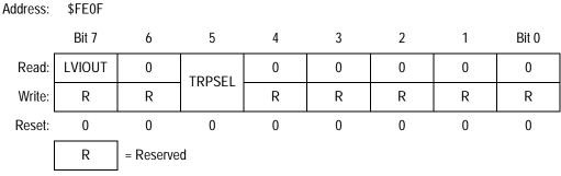
Figure 18-3. LVI Status and Control Register (LVISCR)
