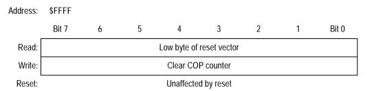
Figure 16-3. COP Control Register (COPCTL)
