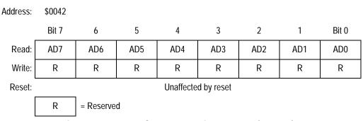
Figure 19-7. ADC Data Register Low (ADRL)
