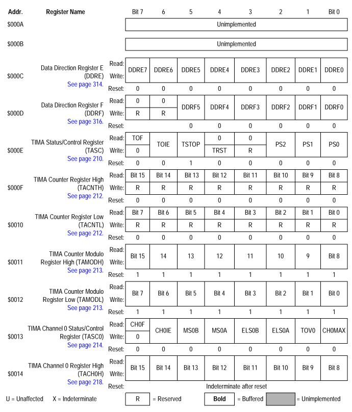
Figure 2-2. Control, Status, and Data Registers Summary (Sheet 2 of 10)
