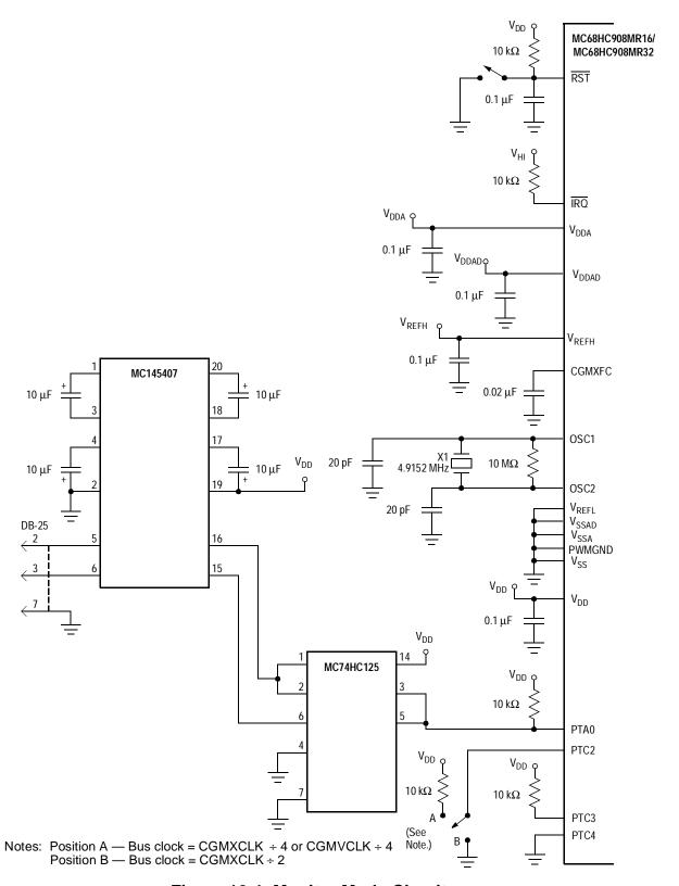
Figure 10-1. Monitor Mode Circuit
