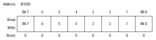
Figure 21-5. Break Address Register Low (BRKL)
