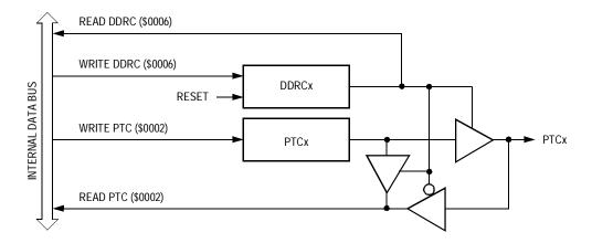
Figure 15-10. Port C I/O Circuit
