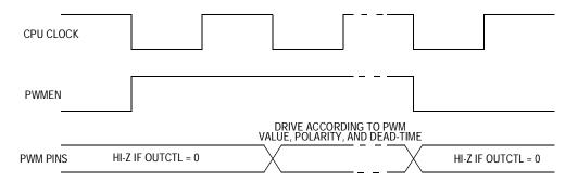
Figure 9-31. PWMEN and PWM Pins
