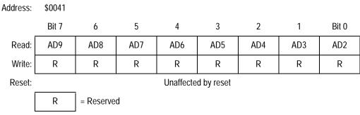
Figure 19-4. ADC Data Register High (ADRH)
