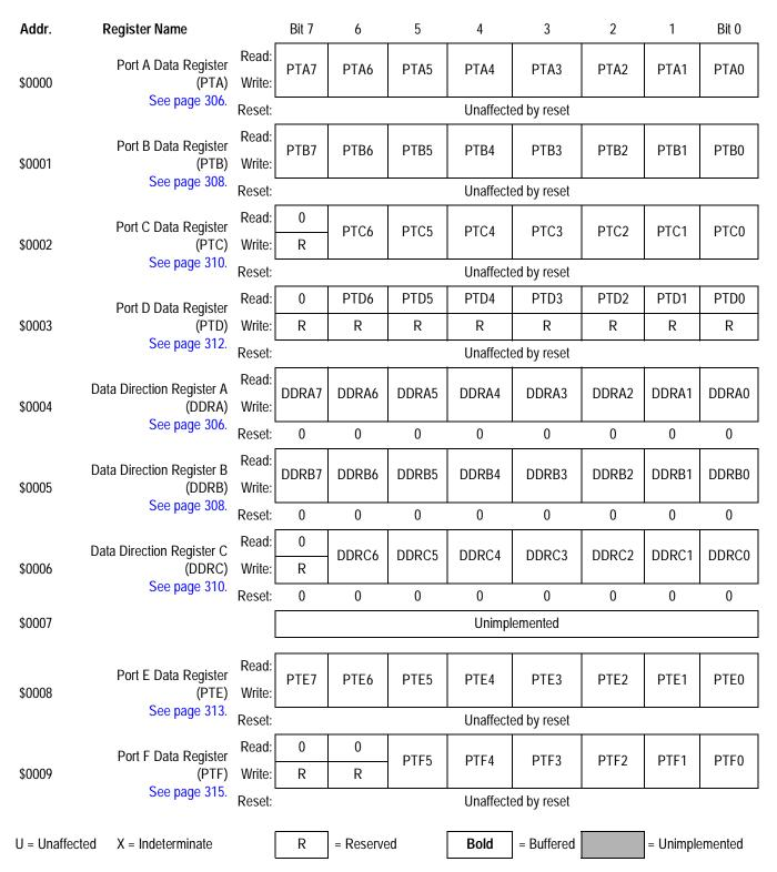
Figure 2-2. Control, Status, and Data Registers Summary (Sheet 1 of 10)
