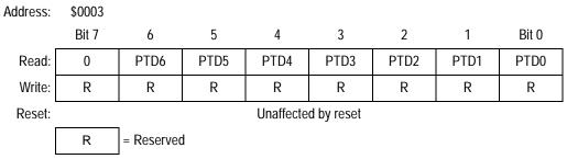
Figure 15-11. Port D Data Register (PTD)
