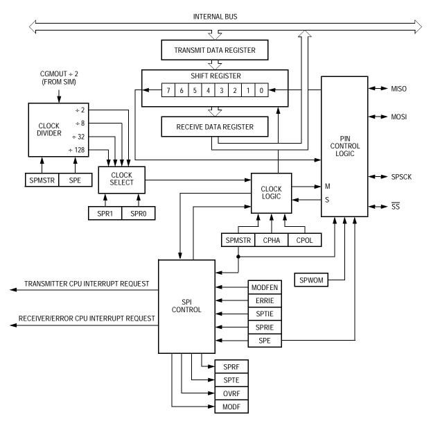
Figure 13-1. SPI Module Block Diagram
