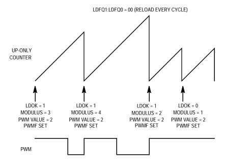
Figure 9-10. Edge-Aligned Modulus Loading
