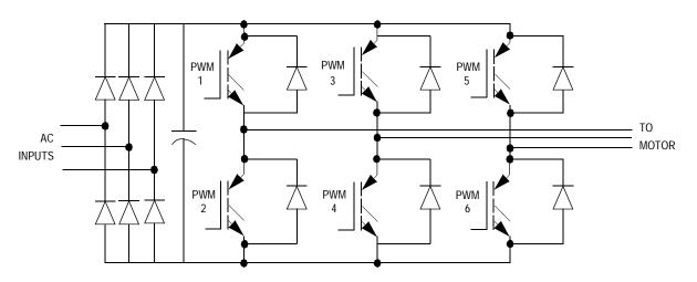
Figure 9-12. Typical AC Motor Drive
