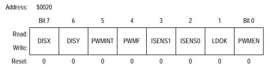
Figure 9-38. PWM Control Register 1 (PCTL1)
