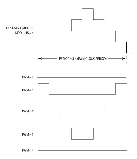
Figure 9-3. Center-Aligned PWM (Positive Polarity)
