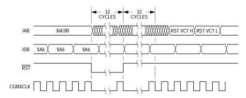
Figure 7-13. Wait Recovery from Internal Reset
