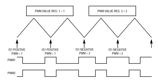
Figure 9-19. Top/Bottom Correction for PWMs 1 and 2
