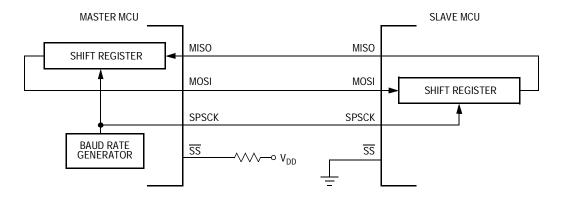
Figure 13-3. Full-Duplex Master-Slave Connections
