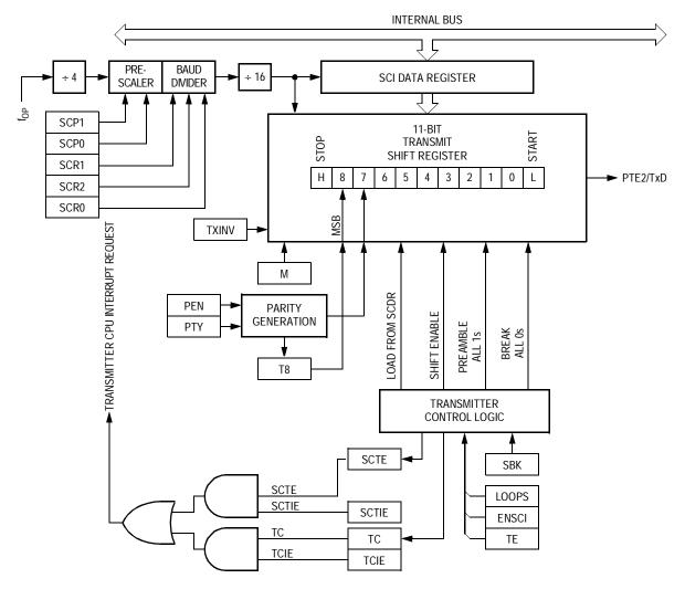
Figure 14-4. SCI Transmitter
