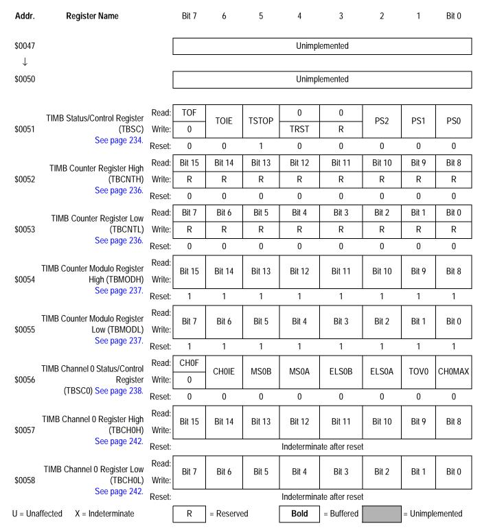
Figure 2-2. Control, Status, and Data Registers Summary (Sheet 8 of 10)
