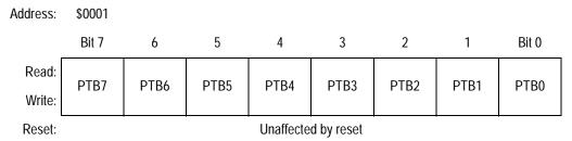
Figure 15-5. Port B Data Register (PTB)
