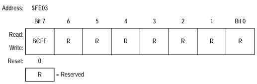
Figure 21-7. SIM Break Flag Control Register (SBFCR)
