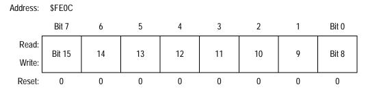
Figure 21-4. Break Address Register High (BRKH)
