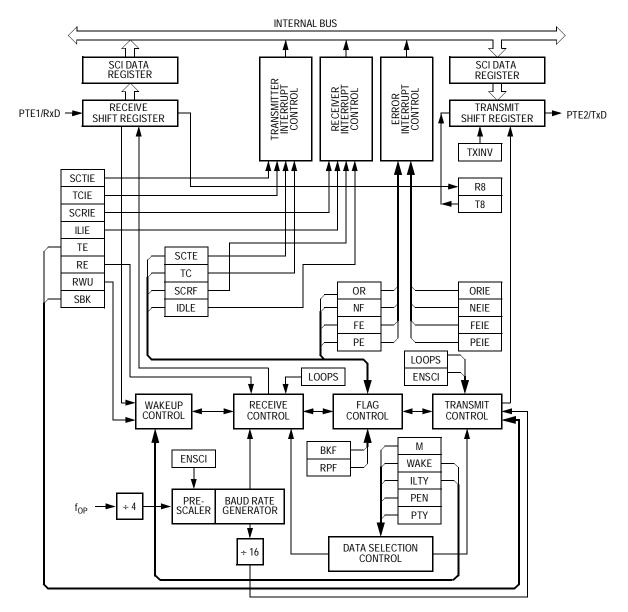
Figure 14-1. SCI Module Block Diagram
