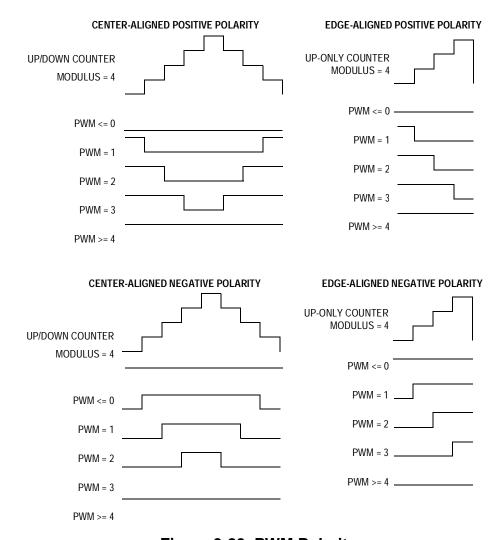
Figure 9-20. PWM Polarity
