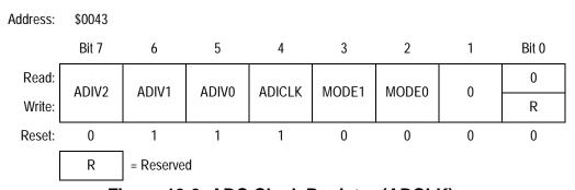
Figure 19-9. ADC Clock Register (ADCLK)
