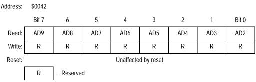
Figure 19-8. ADC Data Register Low (ADRL) 8-Bit Mode
