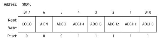
Figure 19-3. ADC Status and Control Register (ADSCR)
