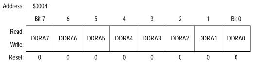
Figure 15-3. Data Direction Register A (DDRA)
