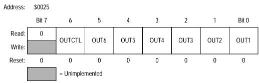
Figure 9-21. PWM Output Control Register (PWMOUT)
