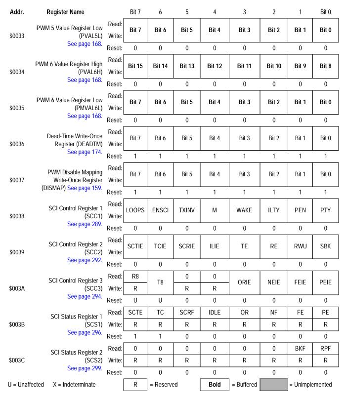
Figure 2-2. Control, Status, and Data Registers Summary (Sheet 6 of 10)
