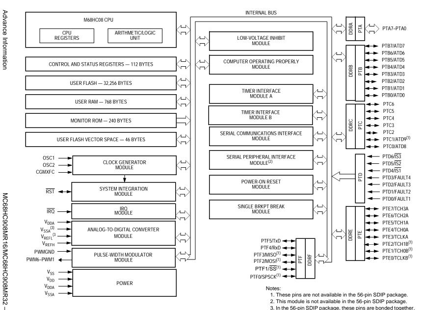
Figure 1-1. MCU Block Diagram
