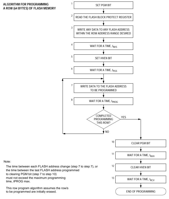
Figure 4-2. FLASH Programming Flowchart
