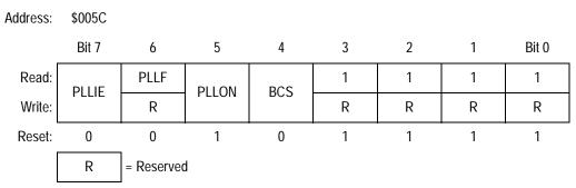
Figure 8-5. PLL Control Register (PCTL)
