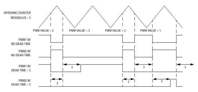
Figure 9-16. Dead-Time and Small Pulse Widths
