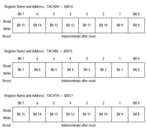
Figure 11-9. TIMA Channel Registers (TACH0H/L-TACH3H/L)
