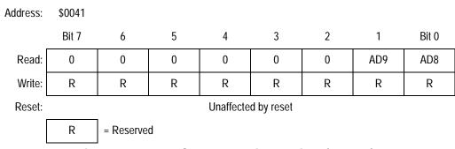
Figure 19-5. ADC Data Register High (ADRH)
