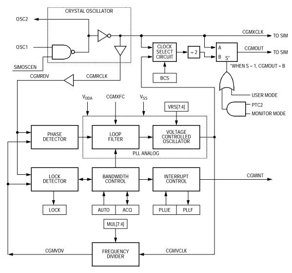
Figure 8-1. CGM Block Diagram
