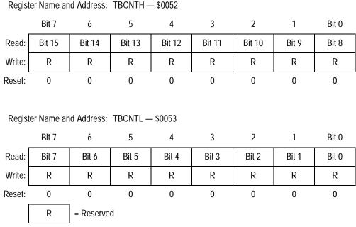
Figure 12-5. TIMB Counter Registers (TBCNTH and TBCNTL)
