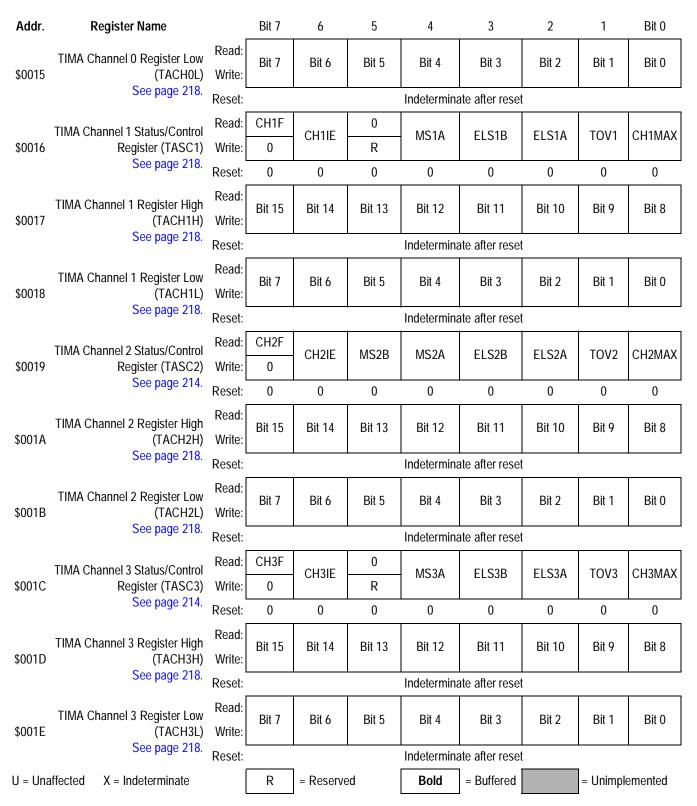
Figure 2-2. Control, Status, and Data Registers Summary (Sheet 3 of 10)
