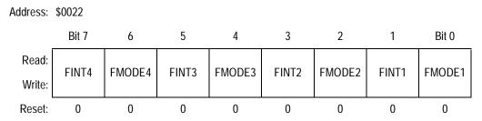
Figure 9-42. Fault Control Register (FCR)
