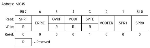
Figure 13-14. SPI Status and Control Register (SPSCR)
