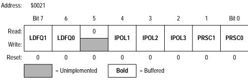
Figure 9-39. PWM Control Register 2 (PCTL2)
