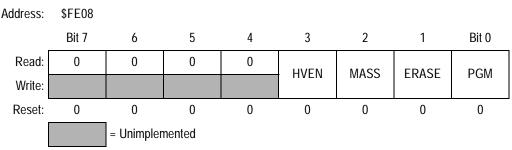
Figure 4-1. FLASH Control Register (FLCR)
