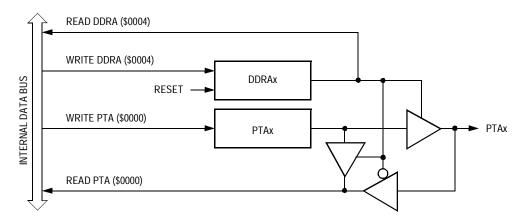
Figure 15-4. Port A I/O Circuit
