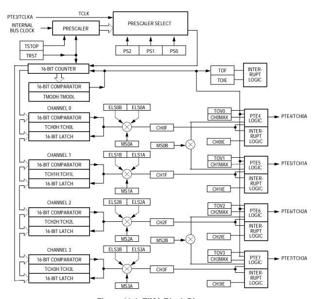
Figure 11-1. TIMA Block Diagram
