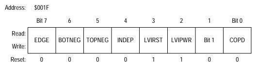
Figure 5-1. Configuration Register (CONFIG)
