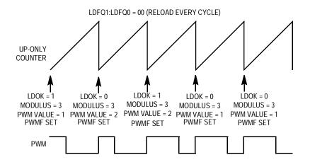
Figure 9-9. Edge-Aligned PWM Value Loading
