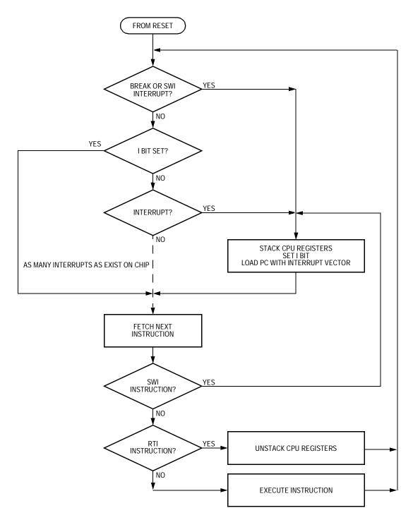
Figure 7-8. Interrupt Processing
