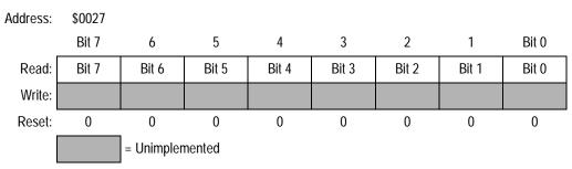
Figure 9-33. PWM Counter Register Low (PCNTL)
