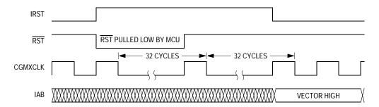
Figure 7-5. Internal Reset Timing
