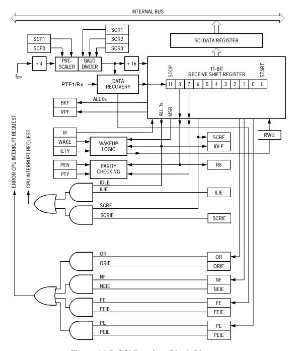
Figure 14-5. SCI Receiver Block Diagram
