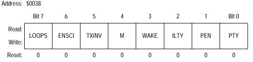
Figure 14-7. SCI Control Register 1 (SCC1)
