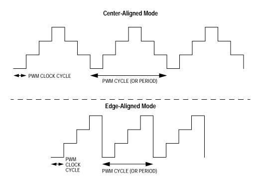
Figure 9-46. PWM Clock Cycle and PWM Cycle Definitions
