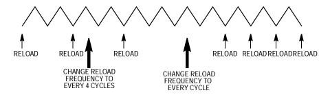
Figure 9-5. Reload Frequency Change
