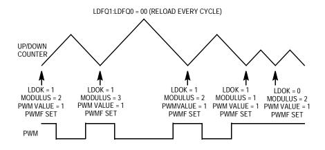
Figure 9-8. Center-Aligned Loading of Modulus
