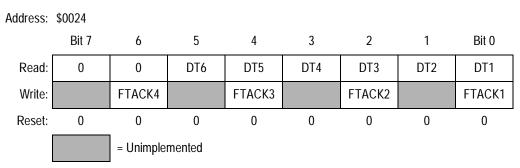
Figure 9-44. Fault Acknowledge Register (FTACK)
