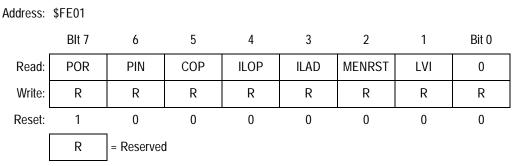
Figure 7-15. SIM Reset Status Register (SRSR)
