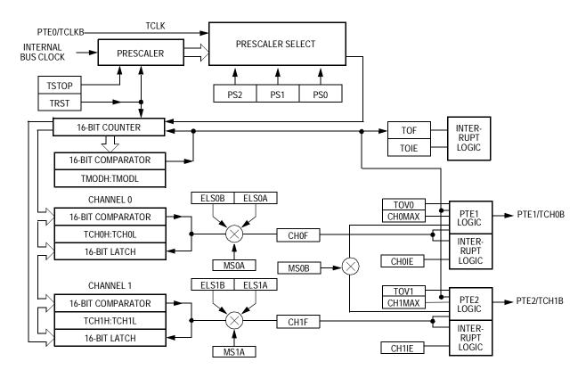
Figure 12-1. TIMB Block Diagram
