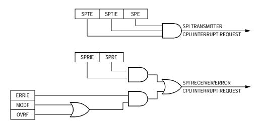
Figure 13-10. SPI Interrupt Request Generation
