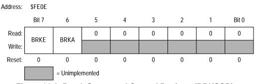
Figure 21-3. Break Status and Control Register (BRKSCR)
