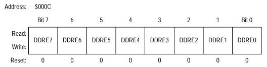
Figure 15-14. Data Direction Register E (DDRE)
