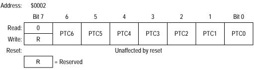
Figure 15-8. Port C Data Register (PTC)
