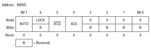
Figure 8-6. PLL Bandwidth Control Register (PBWC)
