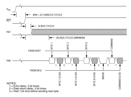
Figure 10-6. Monitor Mode Entry Timing
