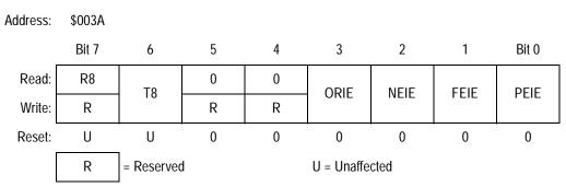
Figure 14-9. SCI Control Register 3 (SCC3)
