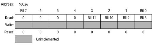
Figure 9-32. PWM Counter Register High (PCNTH)
