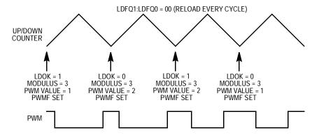
Figure 9-7. Center-Aligned PWM Value Loading
