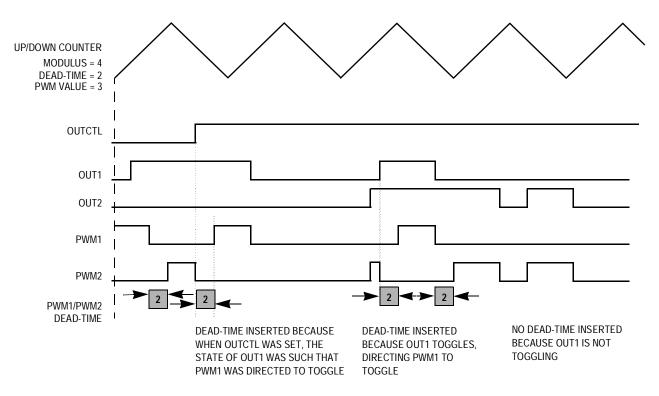
Figure 9-23. Dead-Time Insertion During OUTCTL = 1
