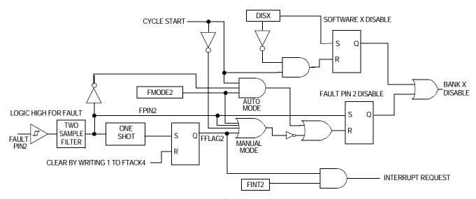
The example is of fault pin 2 with DISX. Fault pin 4 with DISY is logically similar and affects BANK Y disable.
