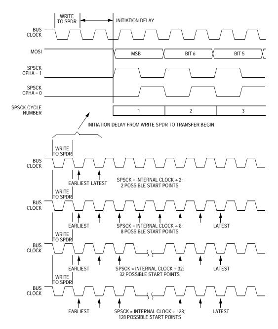
Figure 13-7. Transmission Start Delay (Master)
