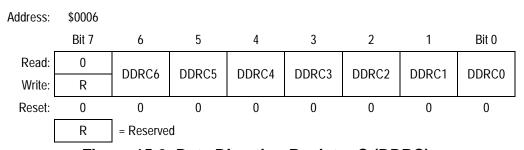
Figure 15-9. Data Direction Register C (DDRC)
