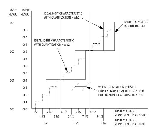
Figure 19-2. 8-Bit Truncation Mode Error
