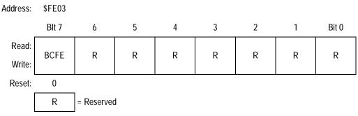
Figure 7-16. SIM Break Flag Control Register (SBFCR)
