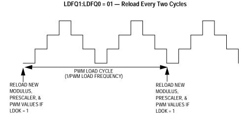
Figure 9-47. PWM Load Cycle/Frequency Definition
