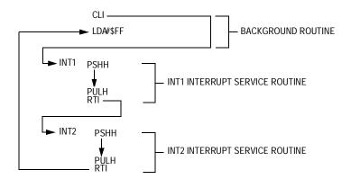
Figure 7-10. Interrupt Recognition Example
