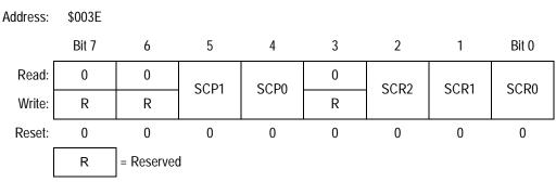
Figure 14-14. SCI Baud Rate Register (SCBR)
