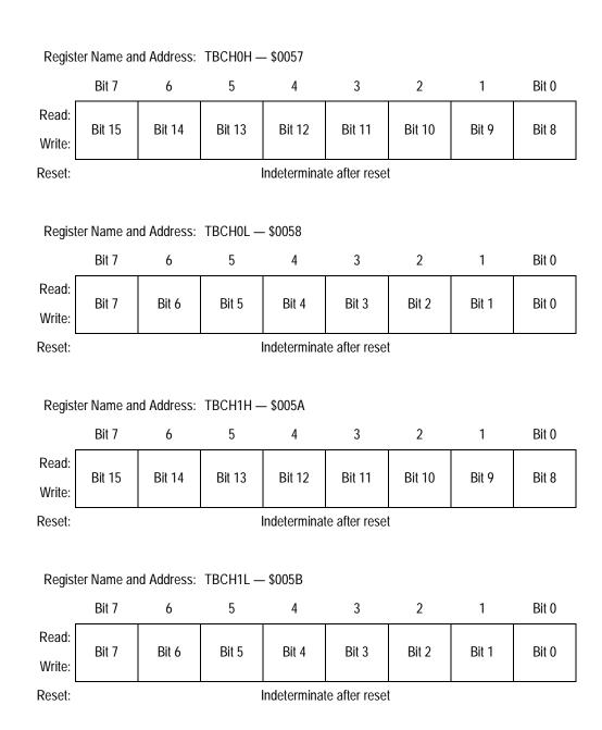
Figure 12-9. TIMB Channel Registers (TBCH0H/L-TBCH1H/L)
