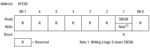
Figure 7-14. SIM Break Status Register (SBSR)
