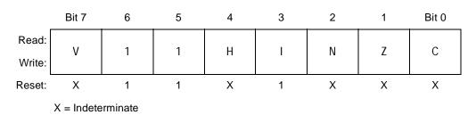
Figure 6-6. Condition Code Register (CCR)
