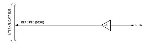
Figure 15-12. Port D Input Circuit
