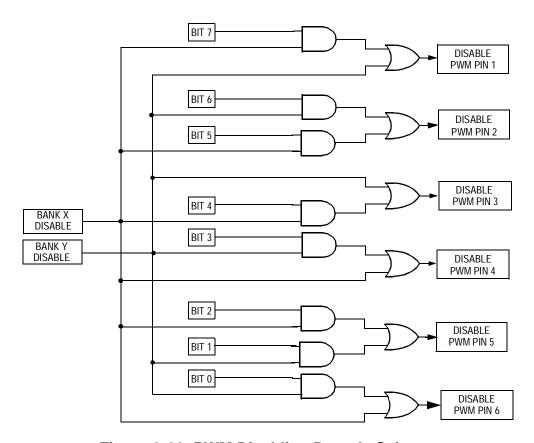
Figure 9-26. PWM Disabling Decode Scheme
