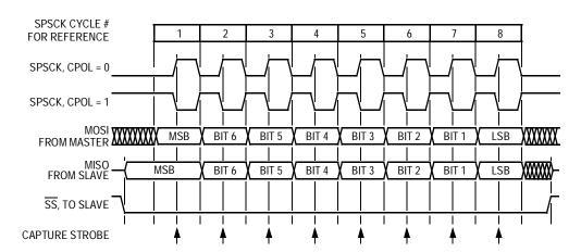
Figure 13-4. Transmission Format (CPHA = 0)
