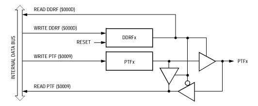
Figure 15-18. Port F I/O Circuit
