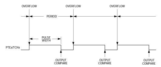
Figure 11-3. PWM Period and Pulse Width
