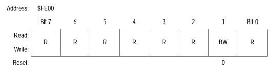
Figure 21-6. SIM Break Status Register (SBSR)
