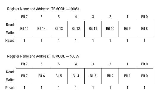
Figure 12-6. TIMB Counter Modulo Registers (TBMODH and TBMODL)
