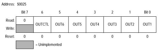
Figure 9-45. PWM Output Control Register (PWMOUT)
