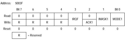
Figure 17-4. IRQ Status and Control Register (ISCR)
