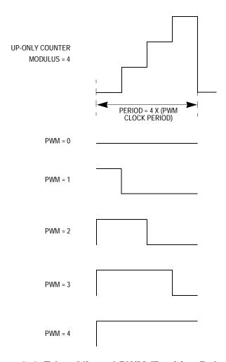
Figure 9-4. Edge-Aligned PWM (Positive Polarity)
