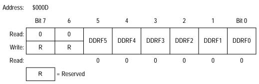
Figure 15-17. Data Direction Register F (DDRF)
