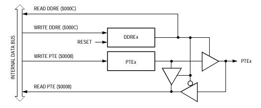
Figure 15-15. Port E I/O Circuit
