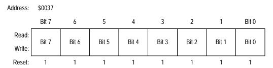
Figure 9-41. PWM Disable Mapping Write-Once Register (DISMAP)
