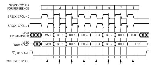
Figure 13-6. Transmission Format (CPHA = 1)
