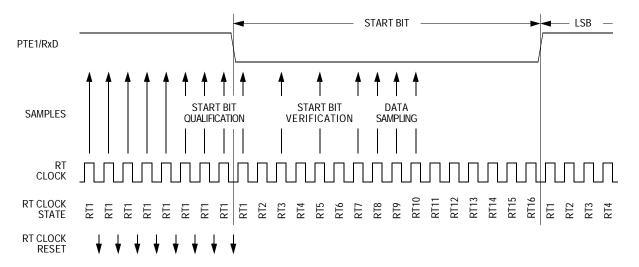
Figure 14-6. Receiver Data Sampling
