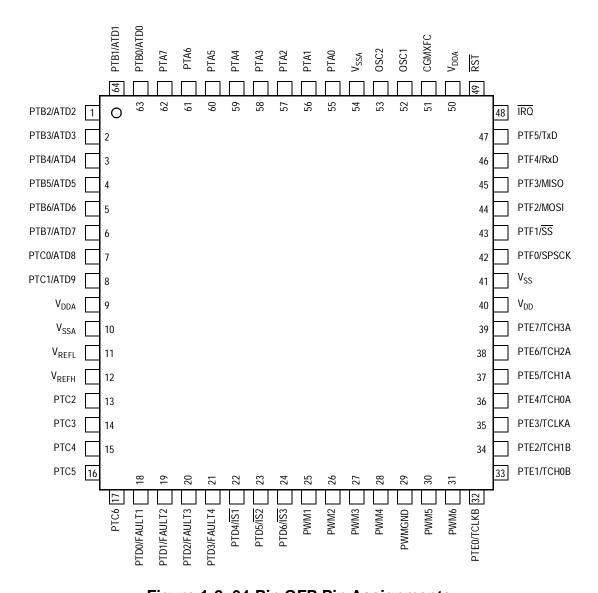
Figure 1-2. 64-Pin QFP Pin Assignments
