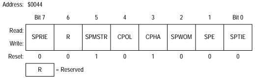
Figure 13-13. SPI Control Register (SPCR)
