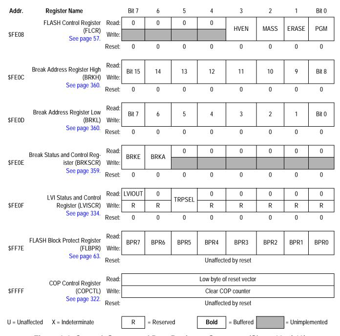
Figure 2-2. Control, Status, and Data Registers Summary (Sheet 10 of 10)
