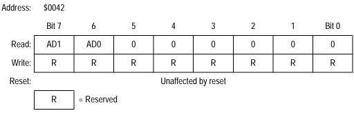
Figure 19-6. ADC Data Register Low (ADRL)
