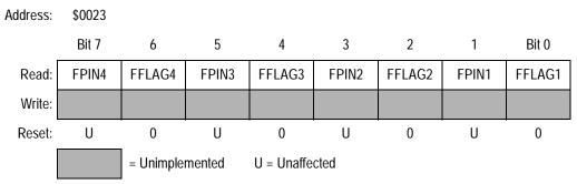
Figure 9-43. Fault Status Register (FSR)
