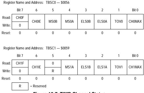
Figure 12-7. TIMB Channel Status and Control Registers (TBSC0–TBSC1)
