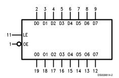
$V_{CC}$  = Pin 20 GND = Pin 10
