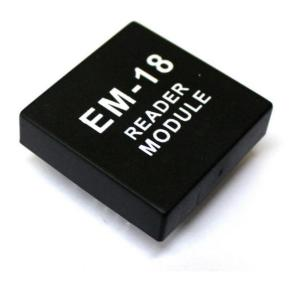
The EM-18 RFID Reader module operating at 125kHz is an inexpensive solution for your RFID based application. The Reader module comes with an on-chip antenna and can be powered up with a 5V power supply. Power-up the module and connect the transmit pin of the module to recieve pin of your microcontroller. Show your card within the reading distance and the card number is thrown at the output. Optionally the module can be configured for also a weigand output.
